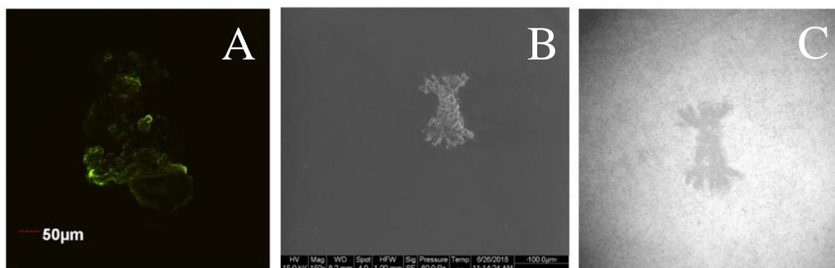
**Figure 27. Correlation of (A) confocal, (B) ESEM, and (C) profilometry on the inlet bottom of Sac 223. There is a large macroscopic deposit seen on the surface. The biologics were not fully degraded from the profilometry image.**
