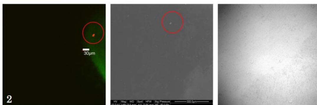
**Figure 51. A small deposit shown by confocal and ESEM on Region 2 of the inlet of Sac 176. The profilometry shows a smooth surface. (34)**
