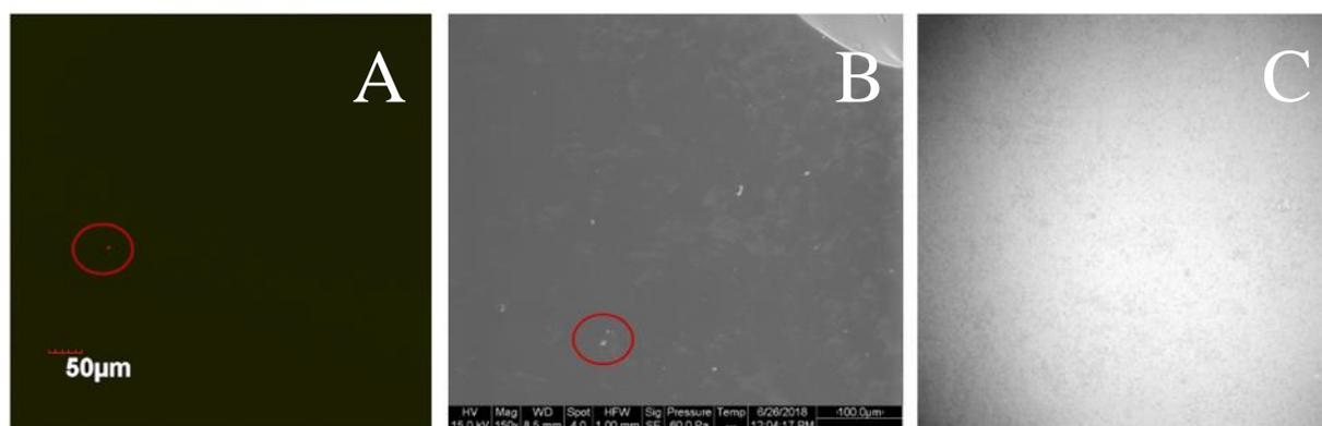
**Figure 29.** Correlation of (A) confocal, (B) ESEM, and (C) profilometry on the outlet top of Sac 223. There is a small, macroscopic deposit shown in the red circles.
