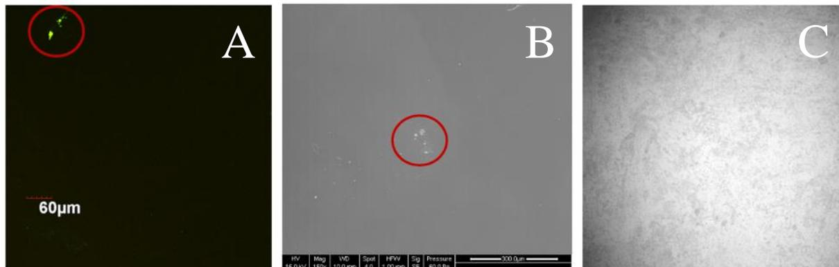
Figure 31. Correlation of (A) confocal, (B) ESEM, and (C) profilometry on the outlet of Sac 240. There is a microscopic deposit shown by the red circles.
