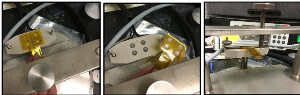
Figure 8: Proper configuration of sensor assembly (steps – left to right)
