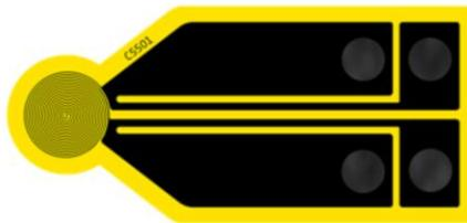
**Figure 7: A sample “Hot Disk Sensor” used by the TPS 500 [30]**
