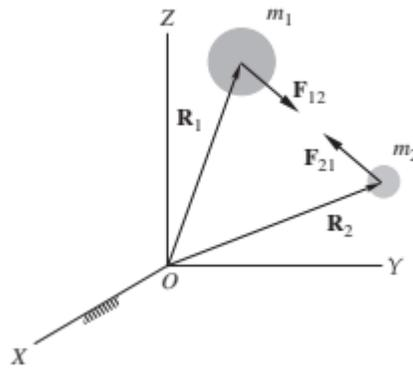
**Figure 2: 2-body Problem with Relative Location and Gravitational Attraction [9]**
