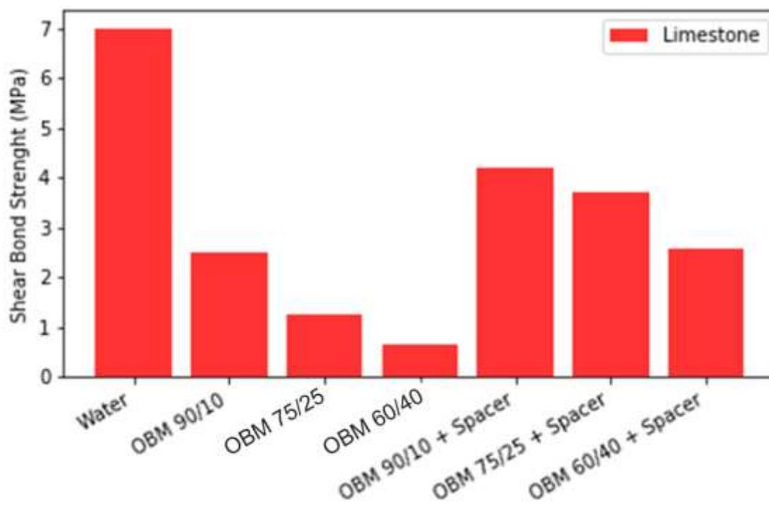
Figure 18. Comparison of shear-bond strengths for different fluid systems in limestone
