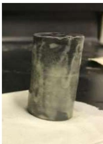
Figure 16. An oil-saturated shale core flushed with spacer
