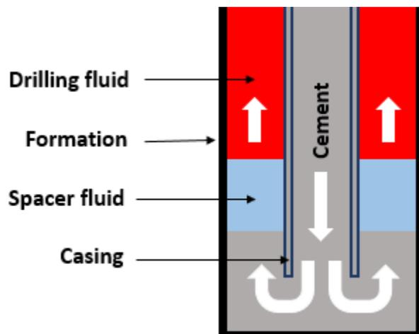
**Figure 1. Schematic of drilling fluid displacement by spacer followed by cement injection**
