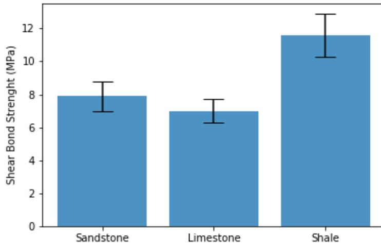
Figure 12. Shear-bond strength values for different water-saturated rocks
