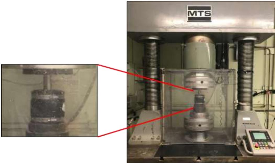
Figure 8. A specimen being tested under axial load frame
