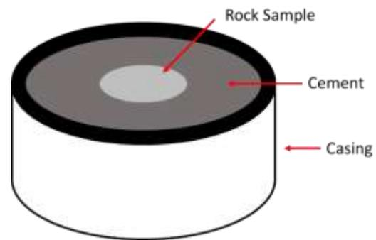
Figure 2. Schematic of a push-out sample
