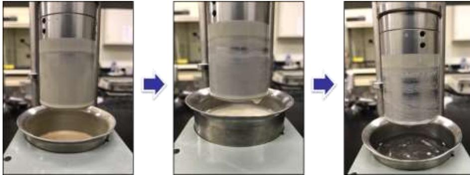
Figure 11. Spacer-OBM compatibility test steps using a rheometer
