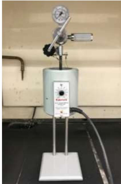
Figure 7. High pressure and high temperature filter press used to saturate rock-cores with OBM
