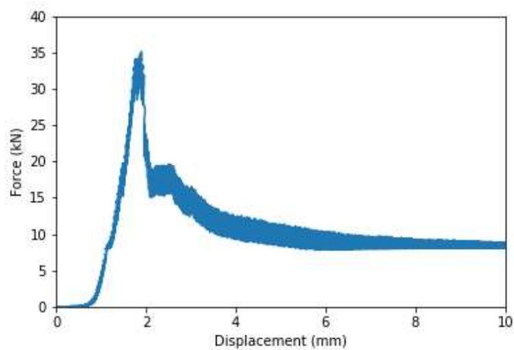
Figure 9. Load vs. Displacement curve for a shale sample saturated in water
