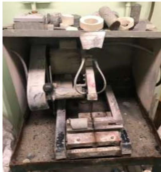
Figure 5. Rock cutting machine
