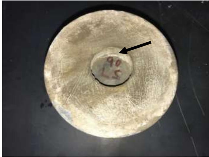
Figure 20. 90/10 OBM-saturated specimen. The arrow shows the mud-cake at the cement-formation interface
