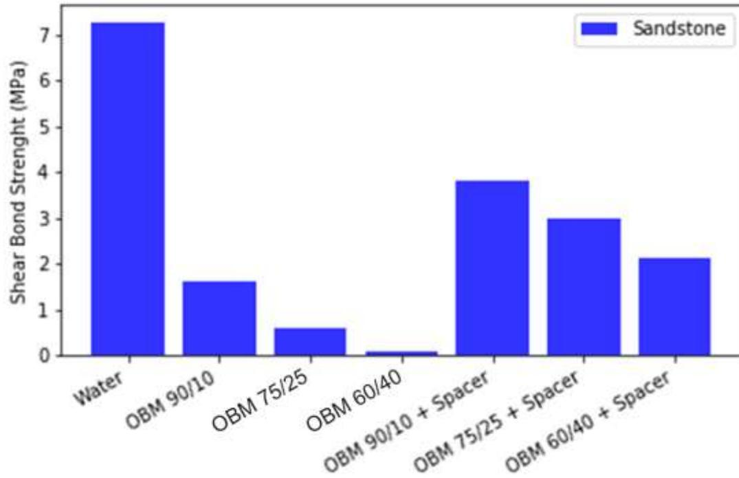
Figure 17. Comparison of shear-bond strengths for different fluid systems in sandstone
