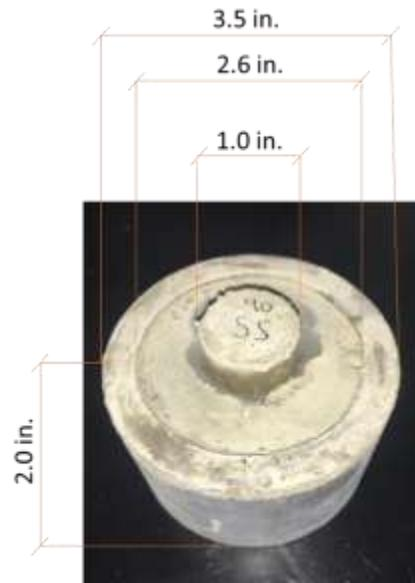
**Figure 6. Specimen dimensions**
