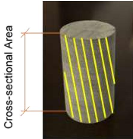
Figure 10. A representation of the rock-cement contact area (the whole circumference area is yellow-dashed)
