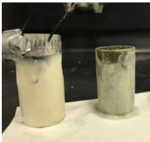
Figure 14. Two rock-cores with different mud-cake thicknesses
