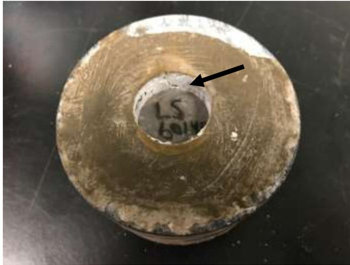
Figure 22. 60/40 OBM-saturated specimen. The arrow shows the mud-cake at the cement-formation interface
