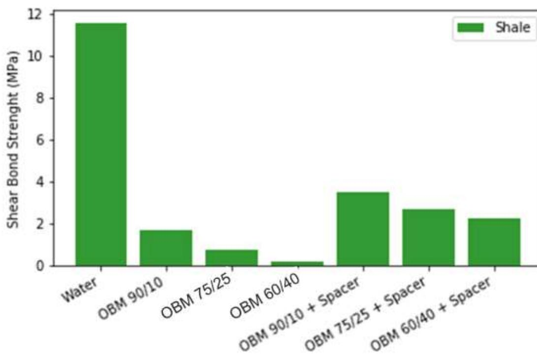
Figure 19 . Comparison of shear-bond strengths for different fluid systems in shale
