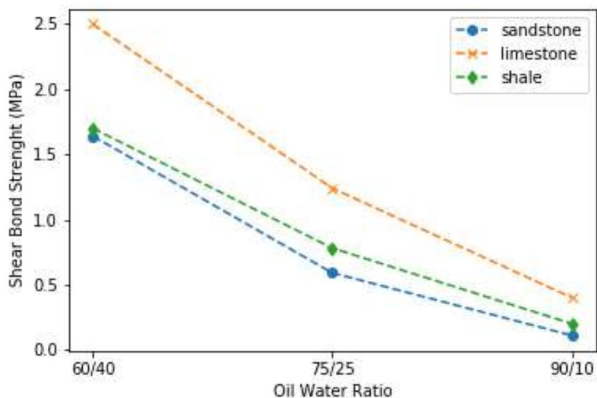
Figure 13. Shear-bond strength values for different oil-saturated rocks
