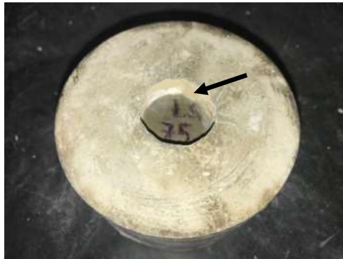
Figure 21. 75/25 OBM-saturated specimen. The arrow shows the mud-cake at the cement-formation interface
