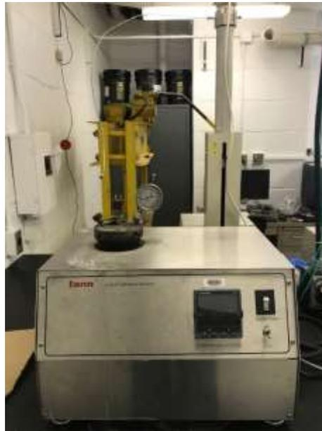
Figure 3. High pressure and high temperature cement curing chamber
