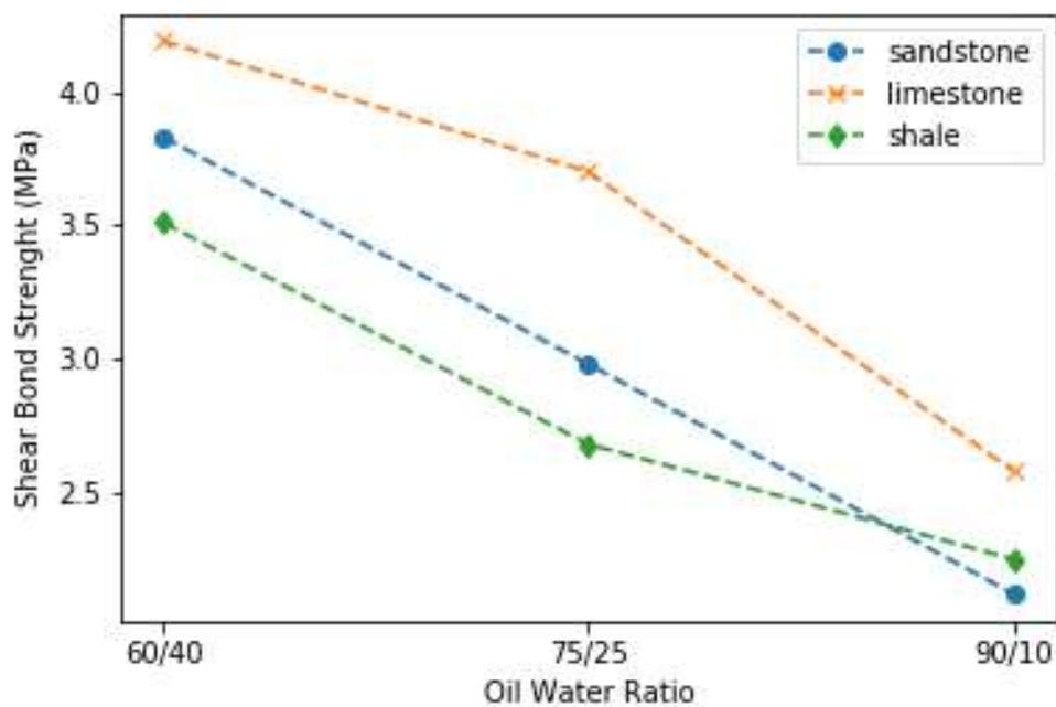
Figure 15. Shear-bond strength values for different oil-saturated rocks flushed with spacer
