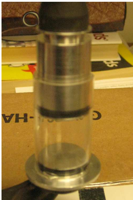
Figure 13: A simple reaction vessel for polymerizing MMA at moderate pressures. The vessel is placed in the mouth of a c-clamp which can be tightened to increase the pressure inside the vessel.
