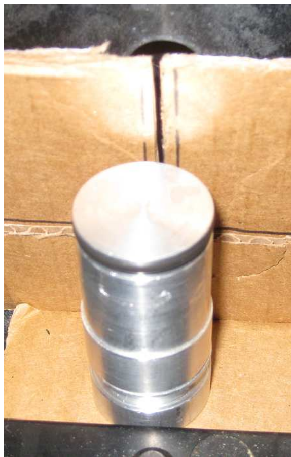
Figure 15: A stand is placed in front of the UV-visible lamp to hold samples at the proper height. A cardboard slit approximately 2mm wide reduces the effects of lensing on the curved surface of the sample.
