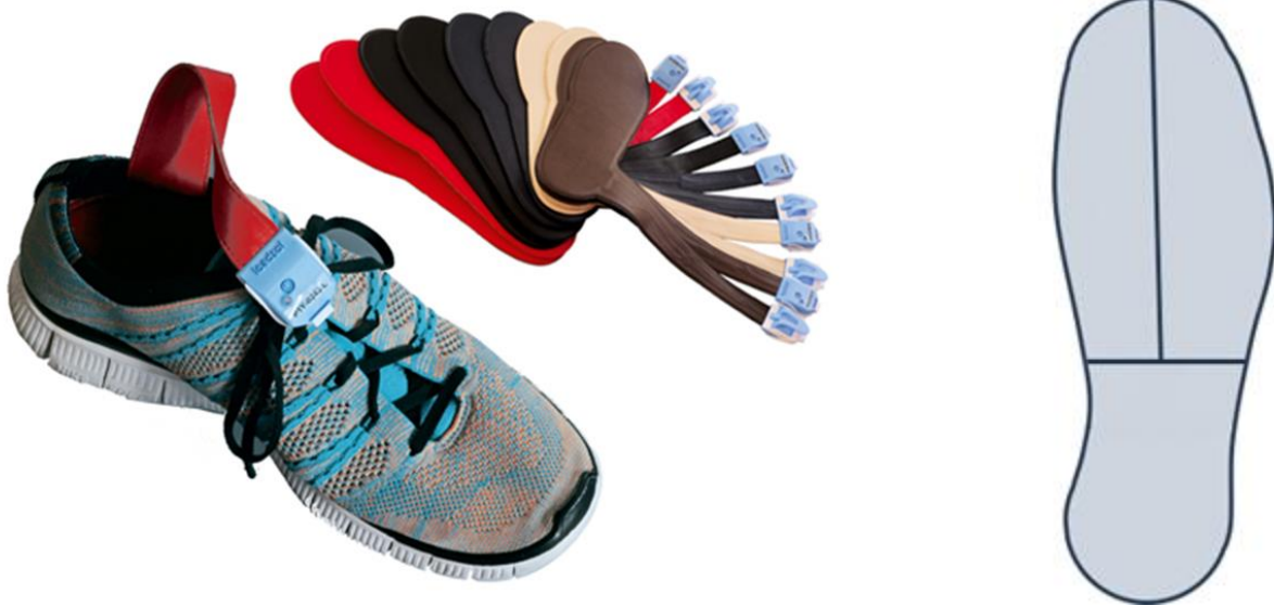
Figure 3.3: Novel© Loadsols® in their five sizes (left), and the configuration of force sensors in the Novel© Loadsols® used in this experiment
