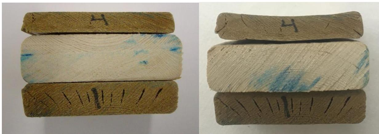
**Figure 3.1:** A) Chemically treated and densified blocks measured against the reference block. B) Same blocks pictured in (A) after an 8-month period.
