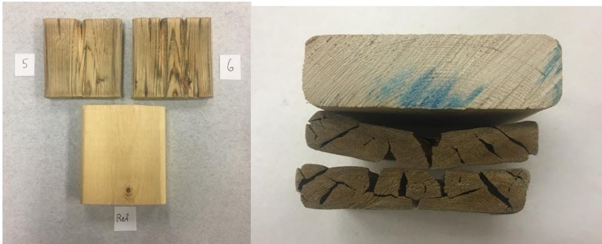
**Figure 3.3:** Chemically treated blocks 5 and 6. Both blocks were exposed to a higher concentration of sodium hydroxide than expected.
