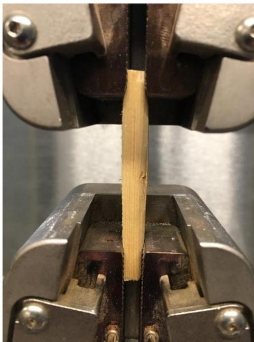
**Figure 2.3:** Untreated spruce wood sample with a thickness of 0.721 cm and length of 6.710 cm clamped in the ASTM D638 tensile strength equipment prior to experimentation.
