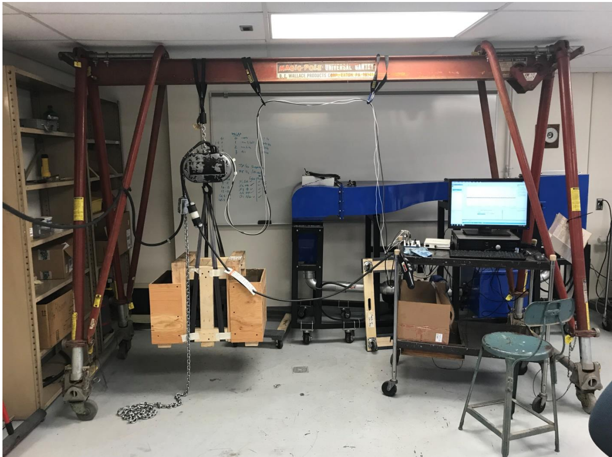
Figure 2: Complete test setup with gantry, motor, weight box, and instrumentation
