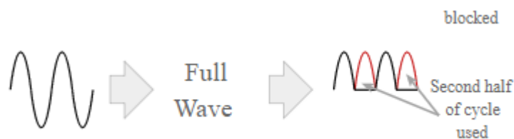
Figure 14: AC to DC conversion through full wave rectifier [7]
