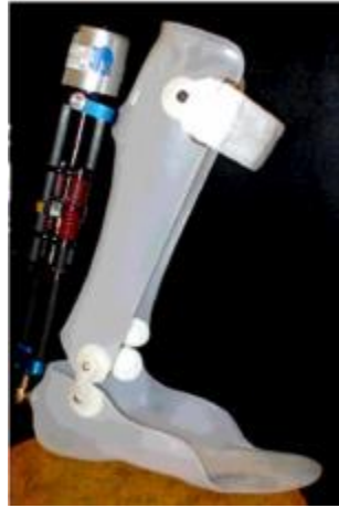
Figure 3: Parallel-limb exoskeleton for torque [9]
