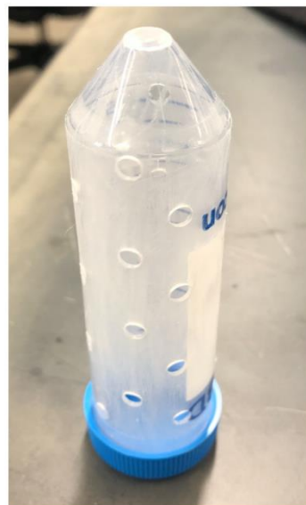
Figure 1: 50mL Conical Tube w/ Ventilation Holes used in the Restraint Study.
