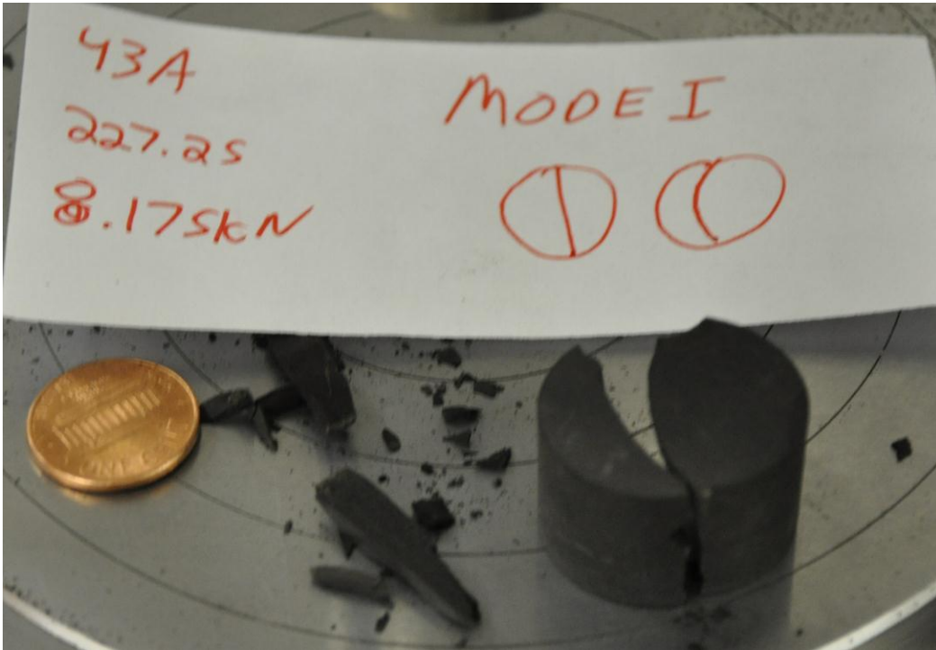
Figure 3-5C: Example of “Off-vertical Mode I” failure. Sample 43A.
