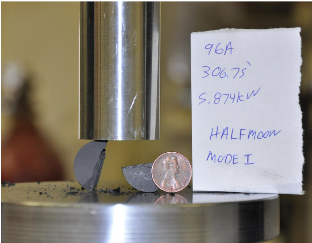
Figure 3-5A: Example of ideal “half moon” Mode I fracture. Sample 96A.
