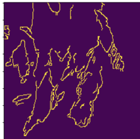
Figure 13 An image of a storm after application of the Canny Edge Detector
