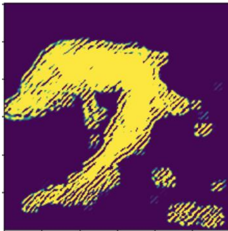
Figure 10 An image following the application of the Gabor filter at a 45 degree angle. This indicates there is a lot of changing texture in the direction.
