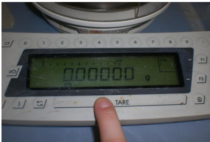
Figure 2-19 Taring of the Sartorius MC210S balance after initial placement of a glass slide
