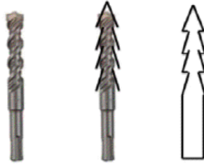
Figure 1-4 2-D simplification of screw design
