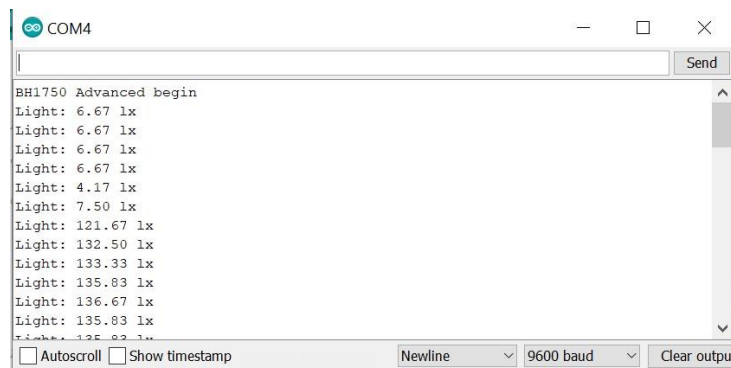
Figure 6. Serial monitor display for the BH1750 light sensor.
