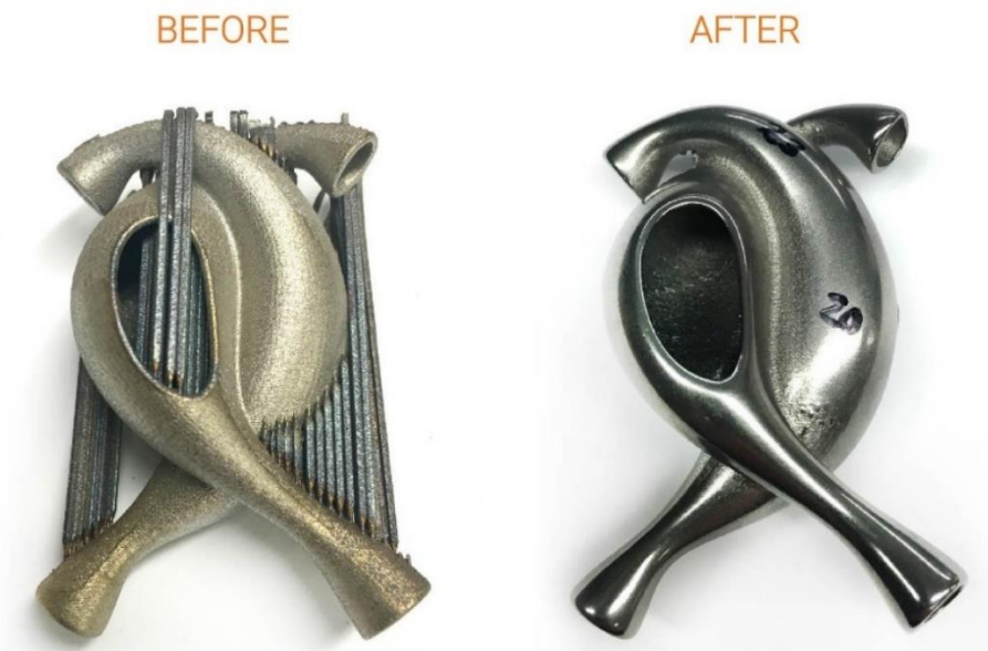
Figure 7. Before and after postprocessing of a 3D printed titanium part [35].
