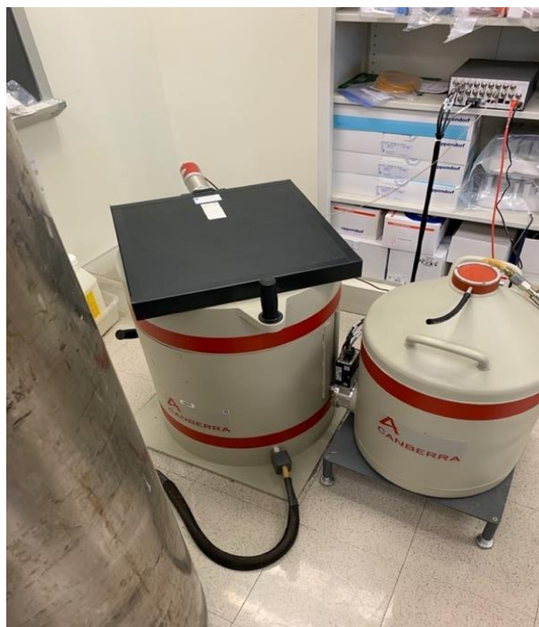
Figure 6: Canberra gamma ray spectrometer in Warner SALTS Laboratory.
