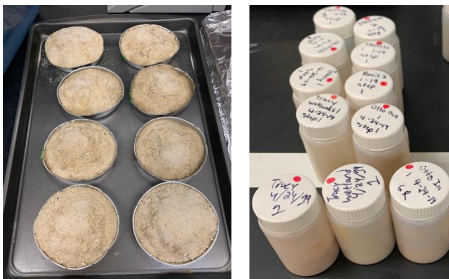
Figure 4: Sediment after being dried in an oven (left). AMD samples packed in 20 mL scintillation vials to be analyzed on a Canberra gamma ray spectrometer (right).
