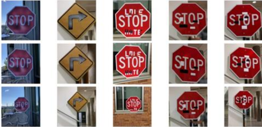
Figure 5. Modified traffic signs disguised as graffiti can be effective adversarial examples (Early, 2019, para.6).
