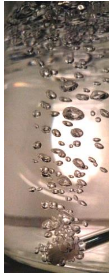
Figure 24: Sparger inserted in the Alginator underneath the flow path to drive flow in the Alginator, supplement the culture with carbon dioxide, and enhance mass transfer by increasing the total surface area of gas-liquid interface.
