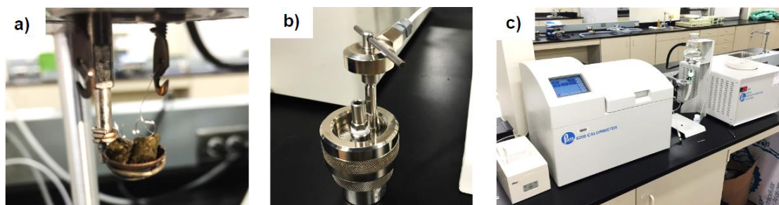
Figure 31: a) Loading of dried C. vulgaris sample. b) Adding oxygen to bomb. c) Parr 6200 bomb calorimeter used.
