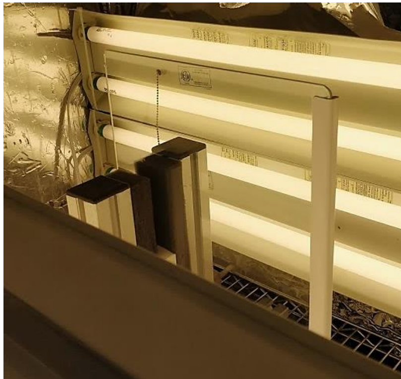
Figure 17: A total of eight fluorescent bulbs (T8, 3500K) were used to provide light to the Alginator. A glass pane was used to simulate the Alginator flow channel for PAR flux analysis.
