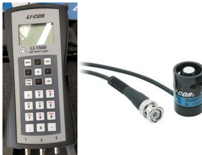
Figure 16: LI-1500 Light Sensor Logger and LI-COR quantum sensor used to measure PAR flux
