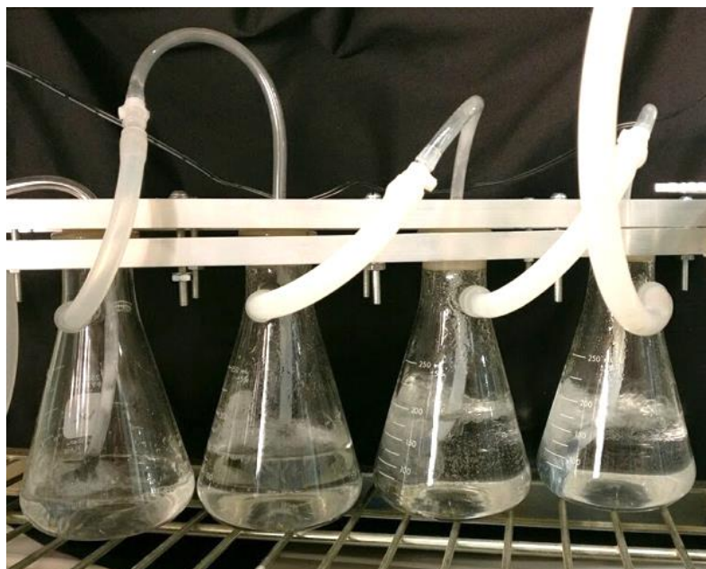
Figure 14: Humidification train to avoid liquid losses during growth.
