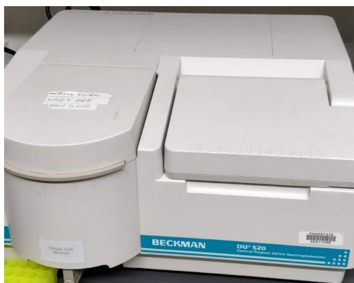
Figure 20: Beckman DU520 spectrophotometer used to measure the optical density of C. vulgaris throughout growth in the Alginator at both 550 nm and 680 nm.
