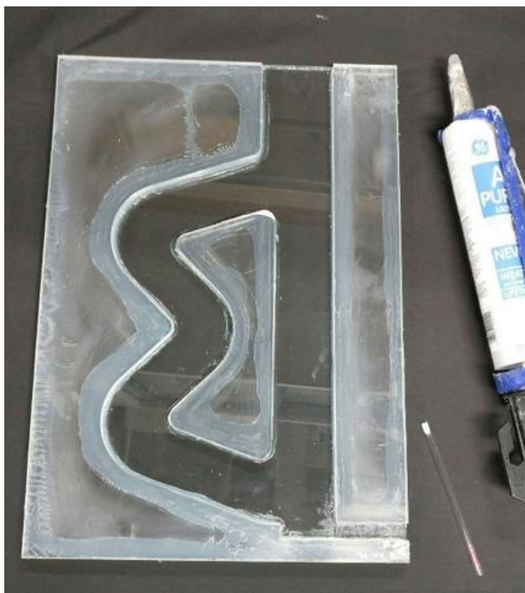
Figure 4: Partially-constructed Alginator with one sheet of glass attached to acrylic, and displaying the silicone caulk with caulking gun and sparger used in the setup.
