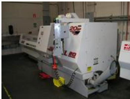
**Figure 17:** Haas SL-20T CNC Lathe [33]
