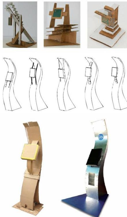
**Figure 25:** Design phases of the DIGI-Net Kiosk [24]
