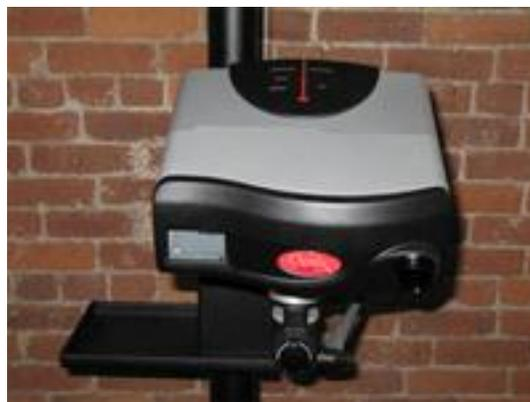
**Figure 24:** Optix 300 3-D Laser Scanner [38]
