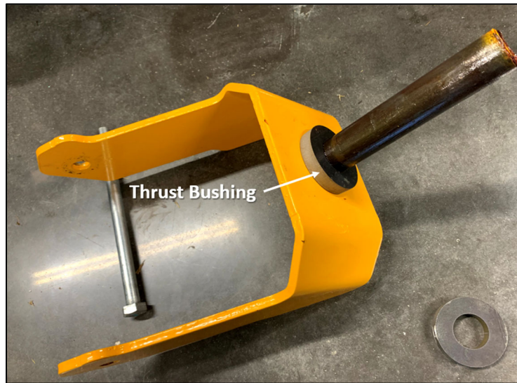
Figure 10.3 - Thrust bushing installed on a caster yoke
