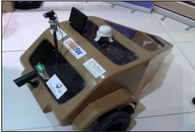
Figure 2.2 – Example of a UGV with multiple sensor inputs [10]
