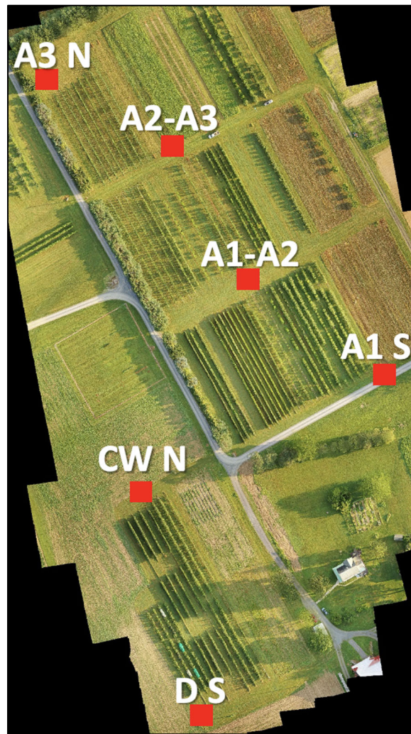
Figure 5.2 – 6 Ground Control Points (GCPs) at Rock Springs Orchard
