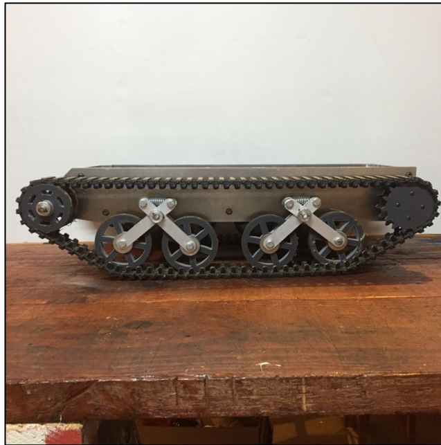
Figure 3.1 - UGV01 left side showing track design
