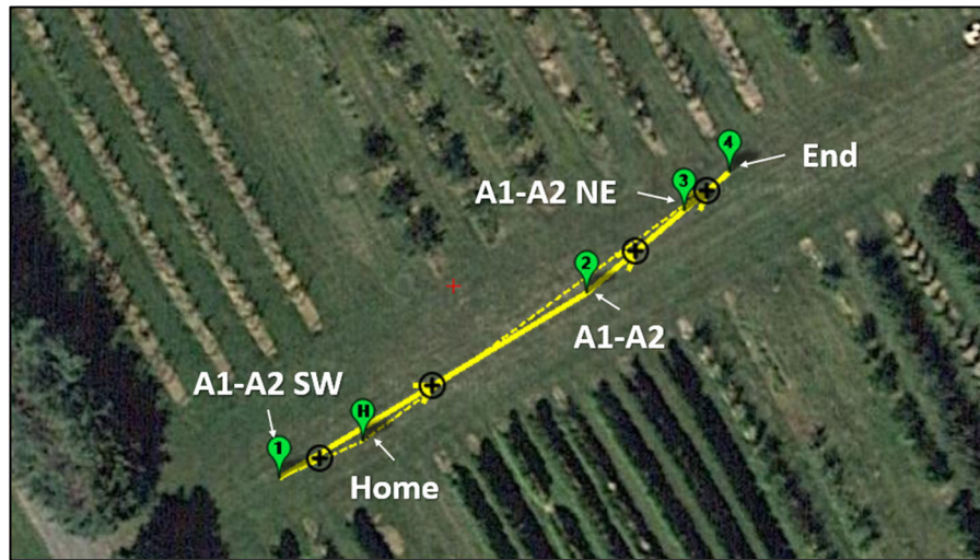
Figure 5.8 - First test track mission displayed in Mission Planner
