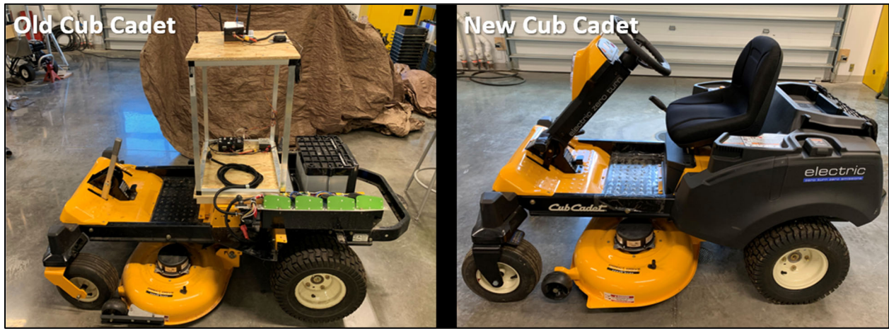
Figure 11.2 - Modified old Cub Cadet compared to the new Cub Cadet
