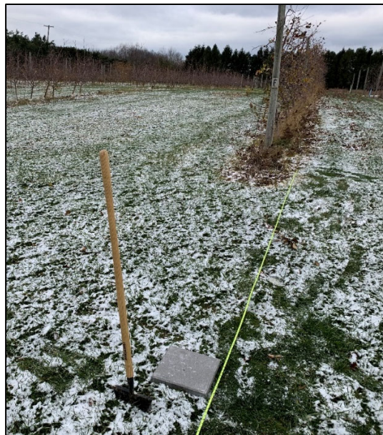
Figure 5.3 – Recessing a stone paver to establish a test track GCP
