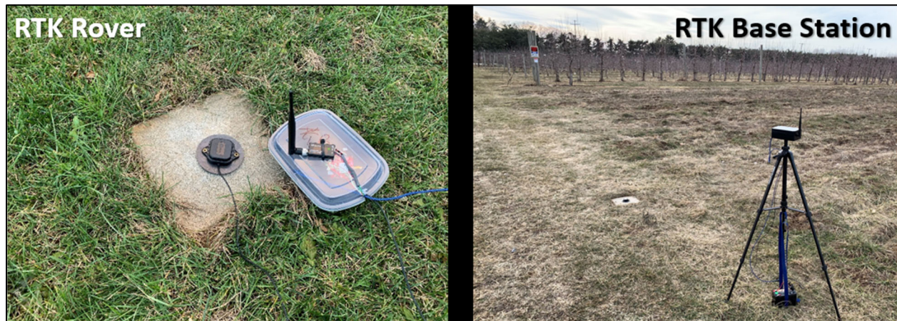
Figure 7.1 - RTK rover (left) and base station (right) equipment during accuracy testing
