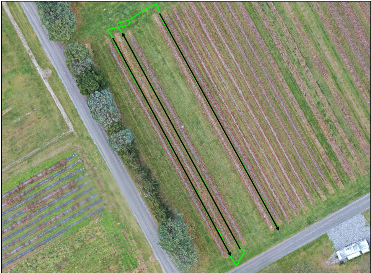
Figure 7.10 - Position trace of UGV01 through orchard block A1
