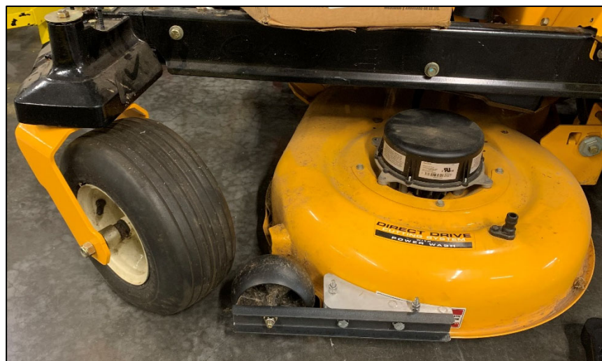
Figure 10.7 - Relocated deck wheel outside sufficiently far from the caster yoke spin radius
