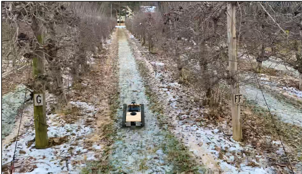
Figure 7.11 - UGV01 navigating a narrow orchard row in block A1
