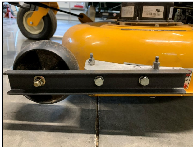
Figure 10.6 – Relocated mowing deck wheel with custom-fabricated mount
