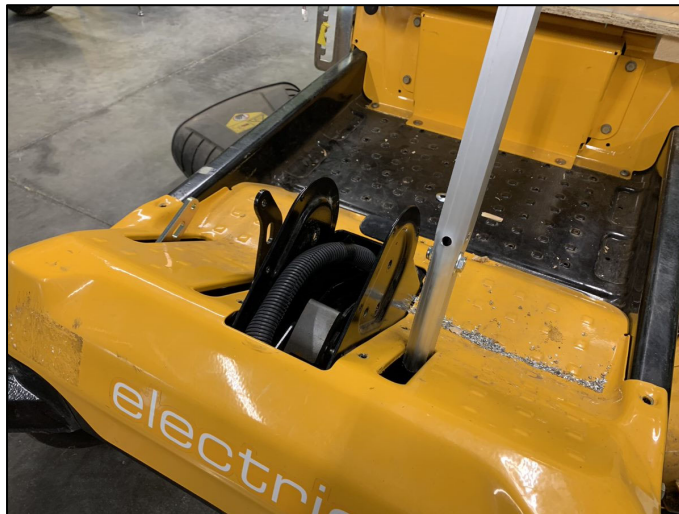
Figure 10.11 - Brake lever bolted to the existing pedal bracket
