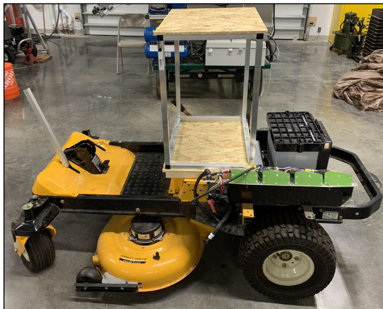
Figure 10.10 - Cub Cadet retrofitted with autonomy platform
