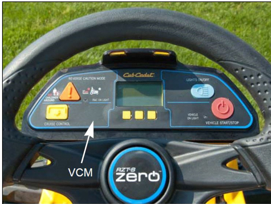
Figure 9.3 - RZT-S Zero Vehicle Control Module (VCM)
