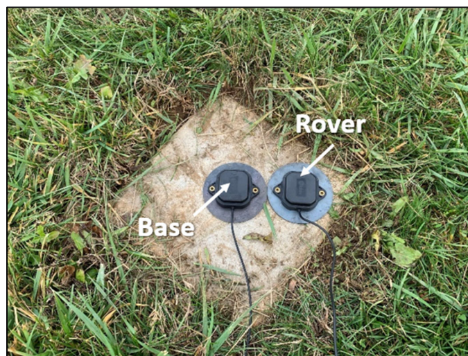
Figure 7.4 - Base and rover GNSS antennas sharing A1 South GCP during testing
