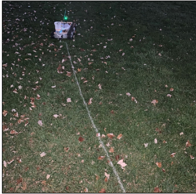
Figure 5.7 - Testing functionality of UGV01 with ground marking device
