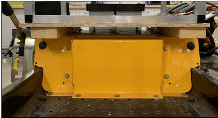
Figure 10.9 – Wooden base of the autonomy platform on the seat deck
