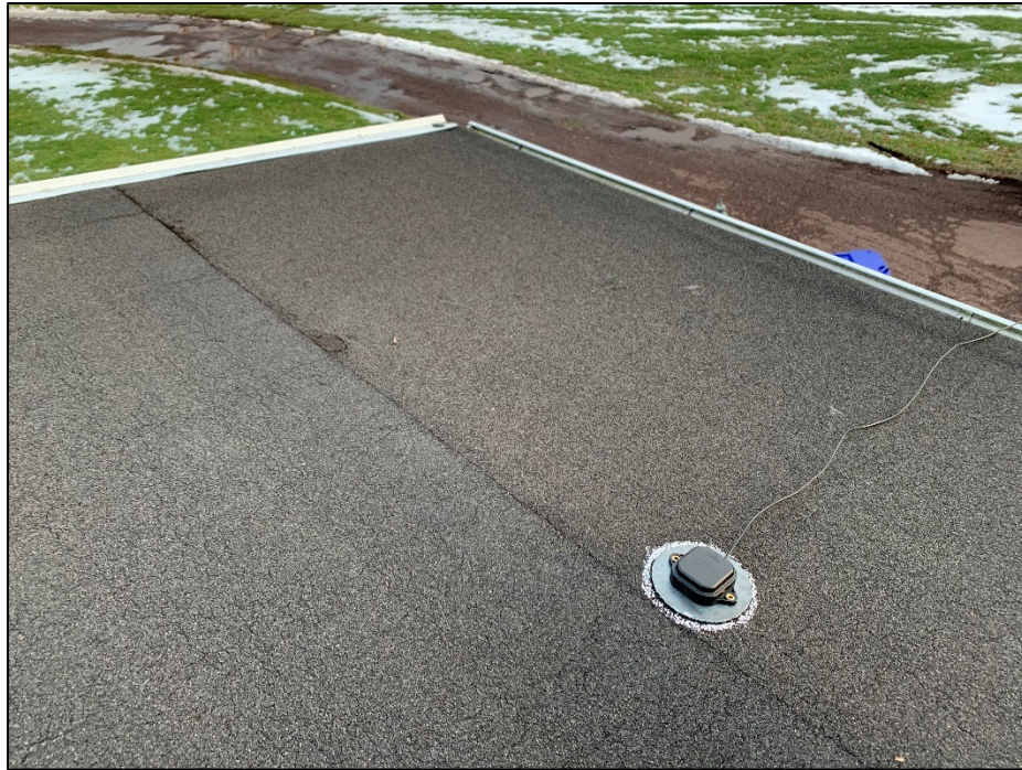
Figure 7.12 - GNSS antenna mounted on roof to determine GCP location
