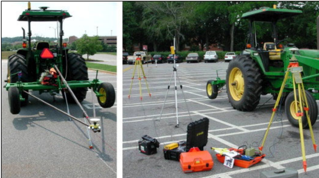
Figure 2.4 - Test rig to record the lateral deviation of an implement [6]
