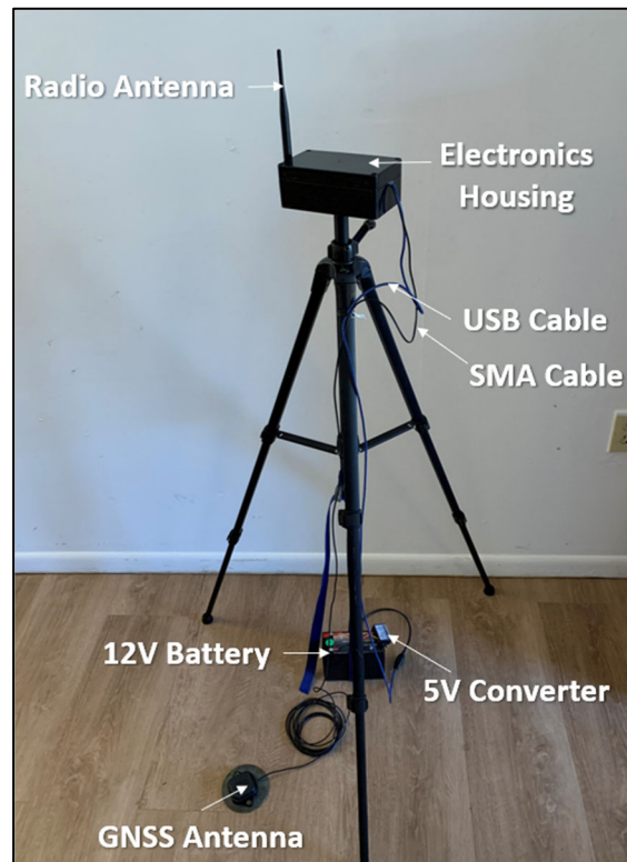
Figure 6.2 - RTK base module assembled with critical components
