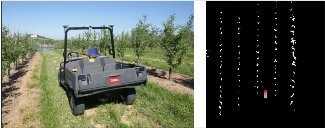
Figure 2.5 – Laser-based autonomous orchard vehicle (left) navigating rows while mapping tree locations (right) [17]
