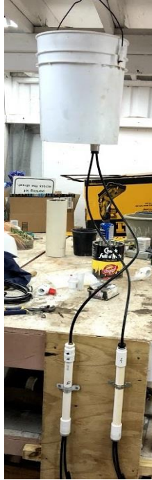
Figure 12. Final column setup with mounted columns attached to drip system
