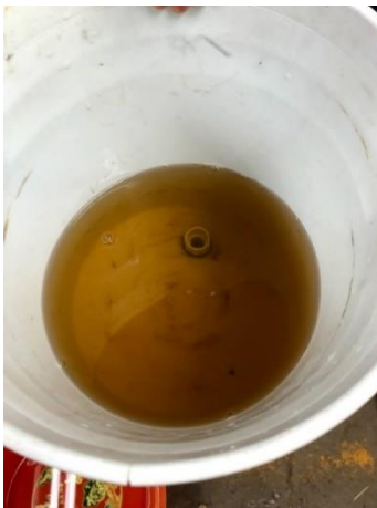
Figure 13. Pond water influent after allowing to settle for 24 hours
