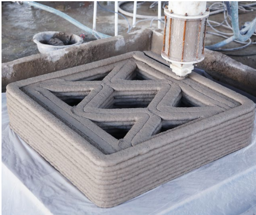
Figure 1. Printing process of concrete components. (Xu, Weiguo et. all, 2020).
