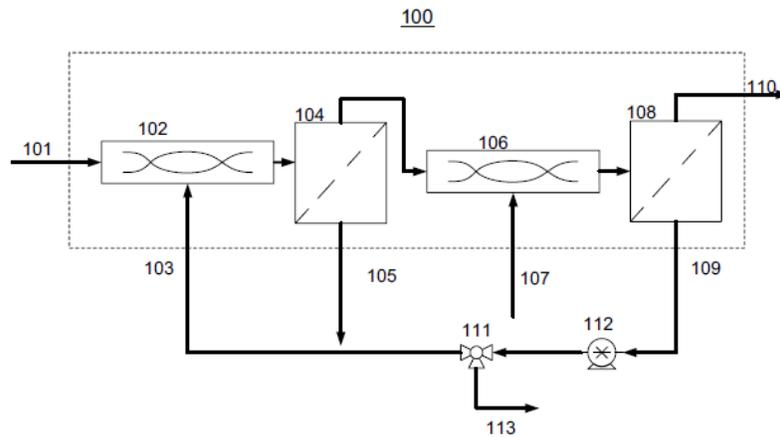
**Figure 2:** Schematic of hollow fiber modules and static mixers in countercurrent tangential flow chromatography. Taken from [11].
