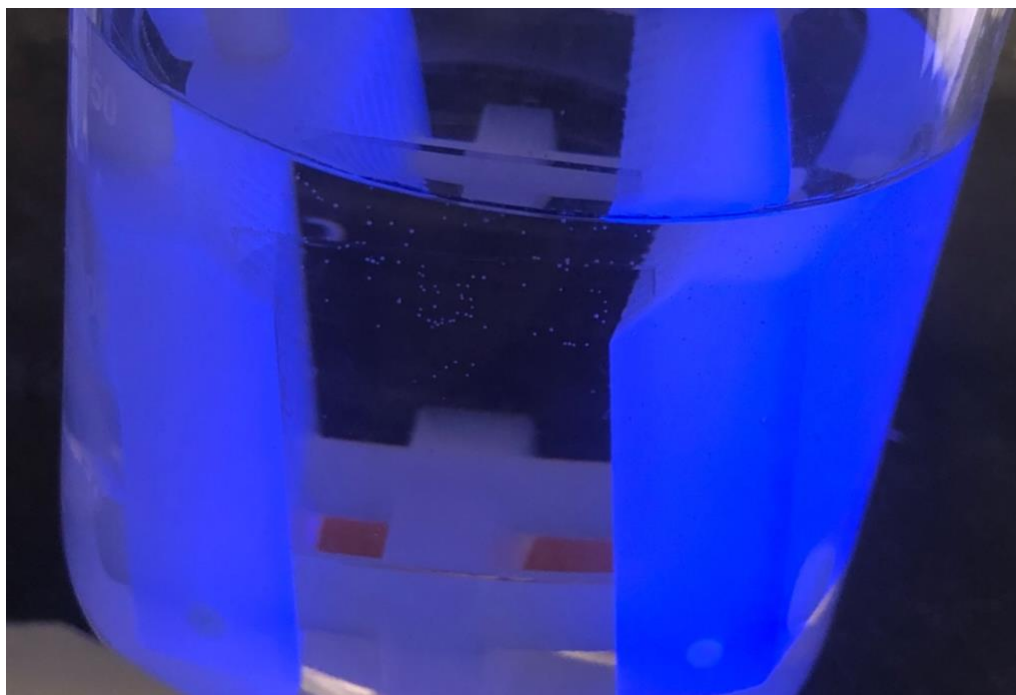
Figure 22: \text{Mn}^{2+} doped ZnSe NPs with MPA and 7 nm ALD and 1.5 nm Pt in Ascorbic Acid under the UV lamp for 30 min.
