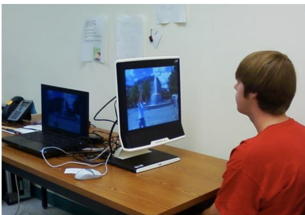
Figure 4: Tobii T60 Eye Tracker System
