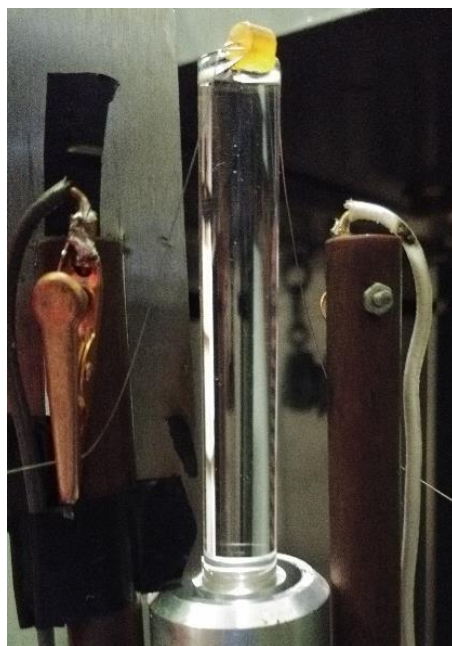
Fig. 14: The sample sits in the strand-holder with the NOSOL/nichrome ignitor [16].
