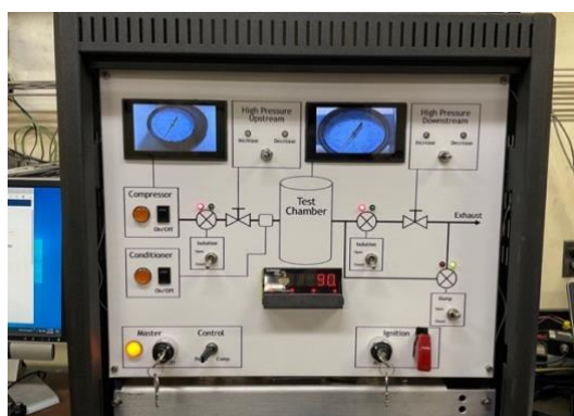
Fig. 10: The LED lights on the panel serve as status indicators
