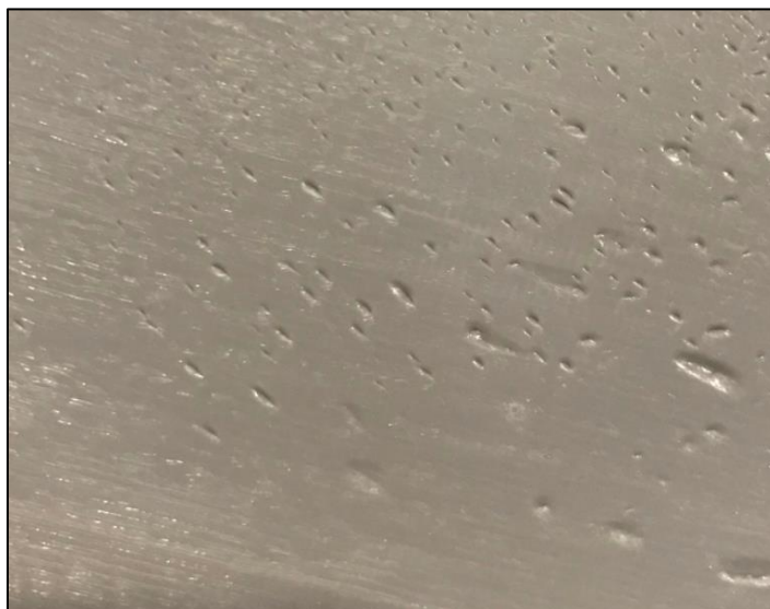
Figure 2: Image of Blemish on Bottom of Food Tray.
