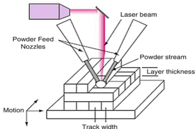
**Figure 3: DED manufacturing process [10]**
