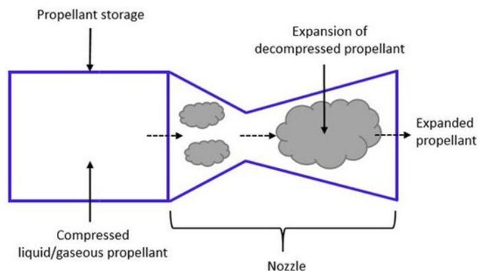
**Figure 5: Diagram of basic resistojet [20]**
