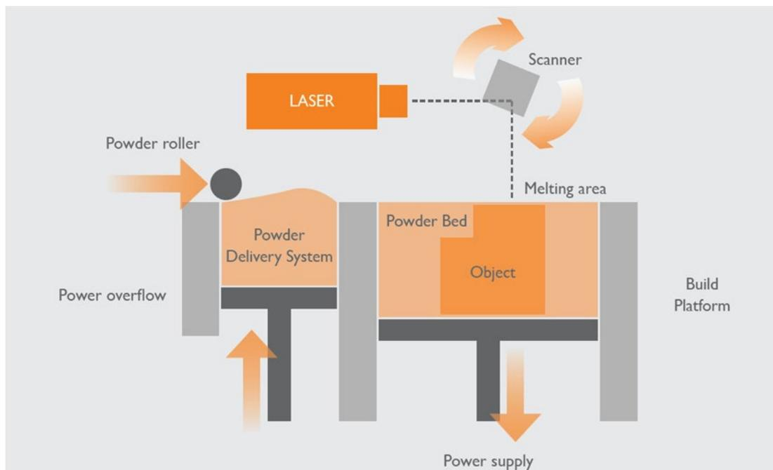
Figure 1: PBF manufacturing process [3]
