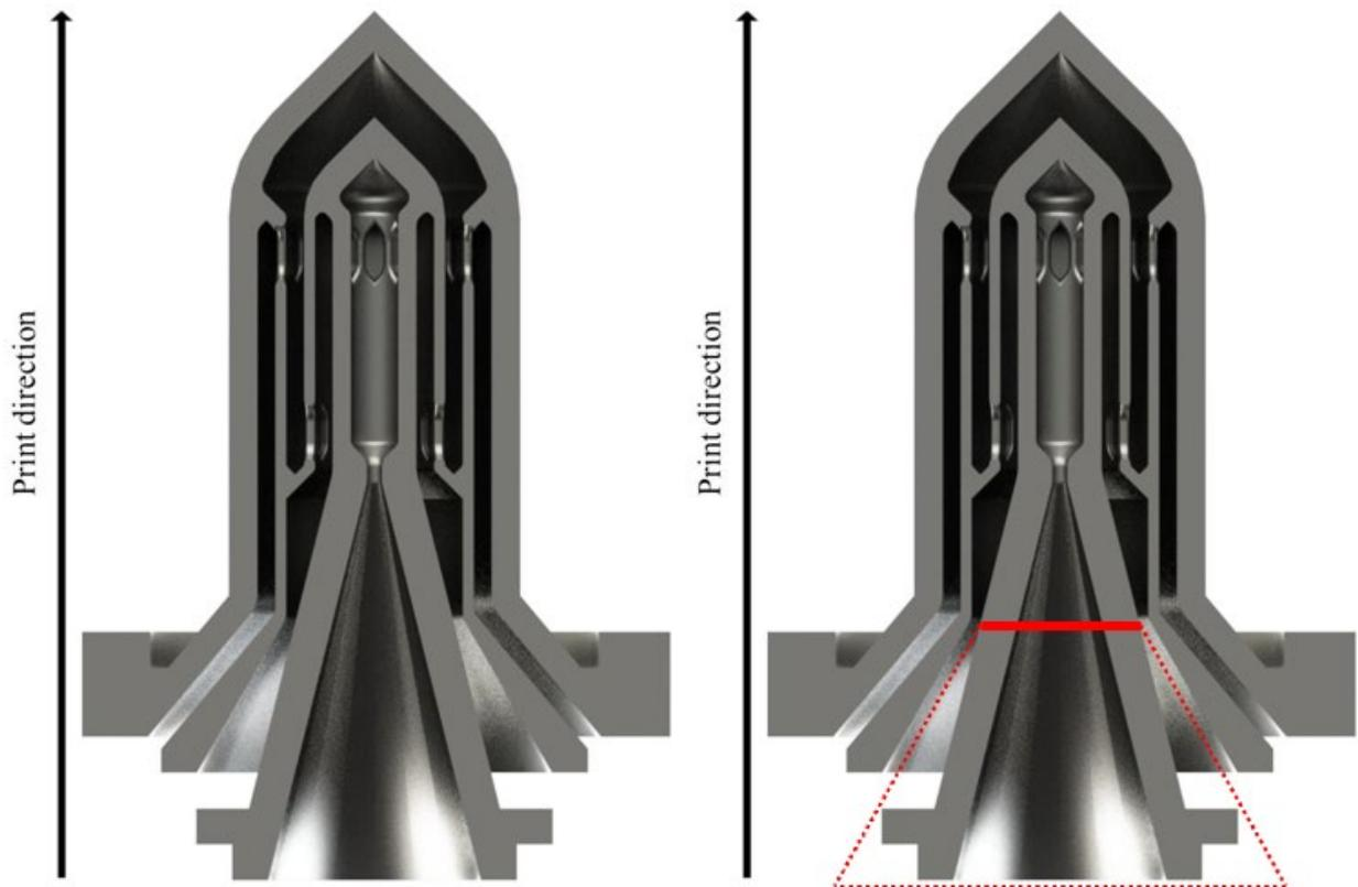
**Figure 7: Single-piece prototype (left) versus two-piece resistojet design (right) [35]**
