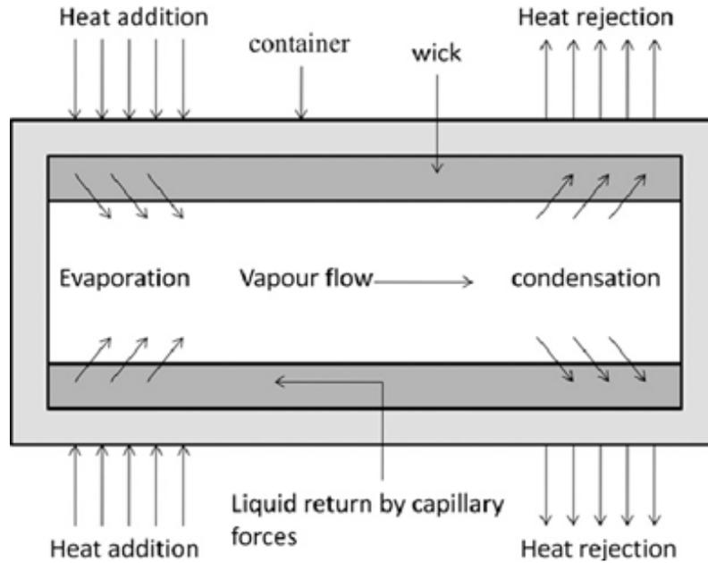
**Figure 4: Diagram of vapor chamber [18]**
