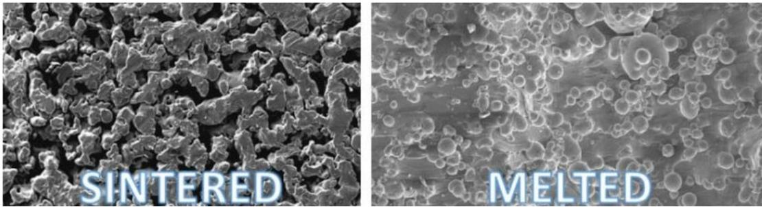
**Figure 2: Sintered metal versus melted metal part structure [5]**
