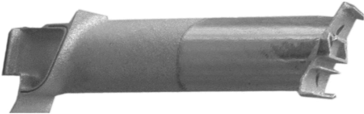
**Figure 6: Low-pressure turbine blade produced with SLM [27]**
