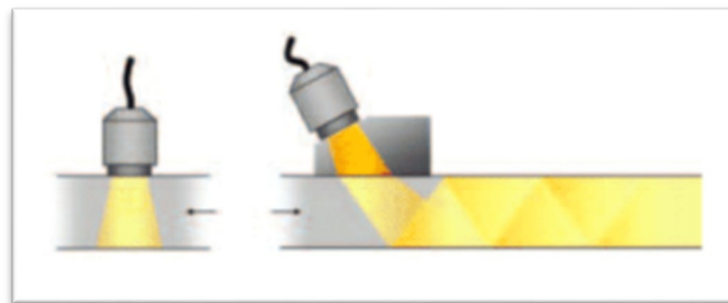
FIGURE 1: PROPAGATION COMPARISON OF BULK VS GUIDED WAVES 8
