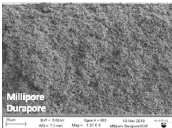
Figure 2: SEM cross section of 0.22 \mu\text{m} PVDF filter highlighting the homogeneous pore size. 9
