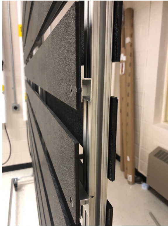
Figure 5. Assembly of plastic slats onto 80/20 frame
