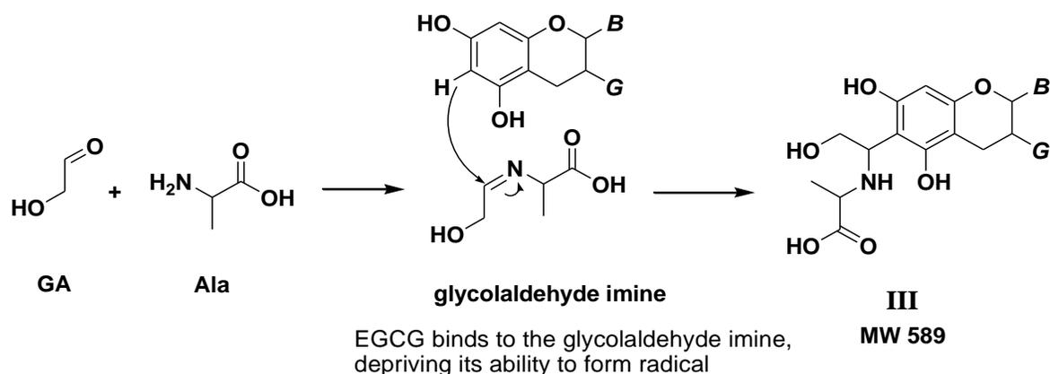
**Figure 3-12.** Proposed mechanism of generation of analyte MW 589 (**III**) and the inhibitory effect of EGCG on the pyrazinium radical formation in GA–Ala model.
