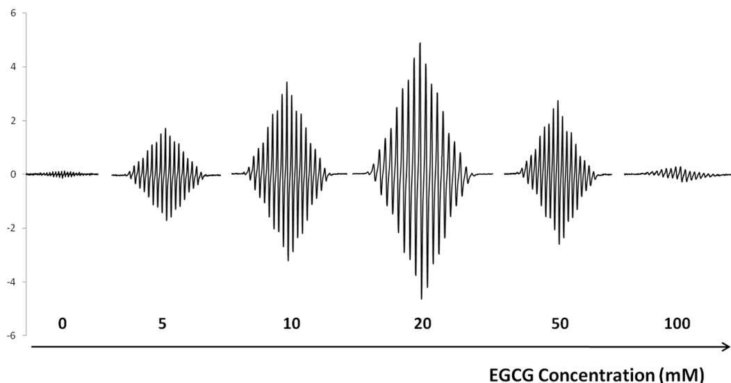
**Figure 3-2.** EPR spectra showing the effect of EGCG on the radical formation in GO-Ala model. For each concentration, the spectrum was selected for its highest intensity along the time-course of changing.
