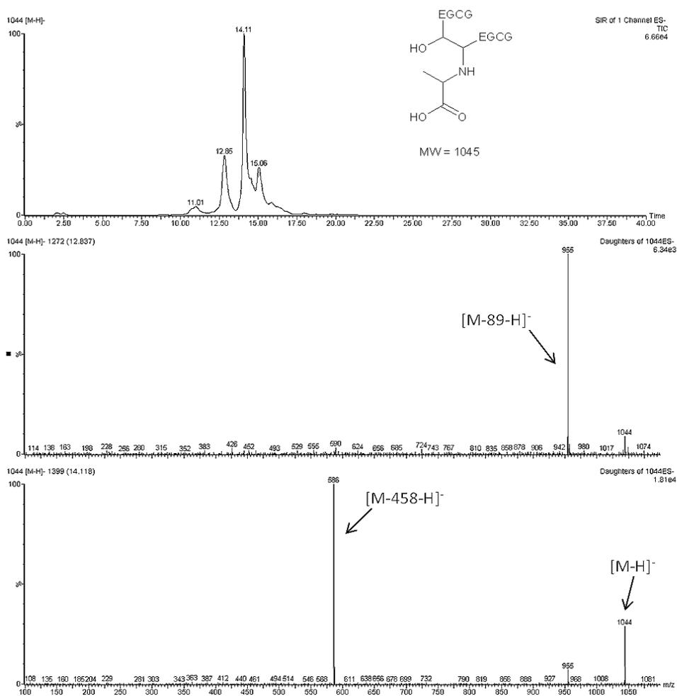
**Figure 3-8.** Chromatograms and LC/MS/MS spectra of analyte MW 1045 (1044 [M-H]<sup>-</sup>) generated from GO-Ala-EGCG model. The EGCG concentration was at 100 mM.
