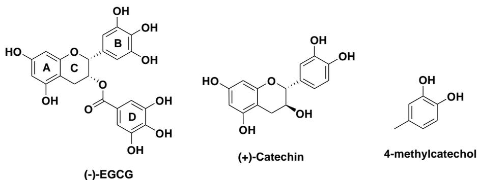
**Figure 3-3.** Structures of (-)-EGCG, (+)-catechin, and 4-methylcatechol used in this study.
