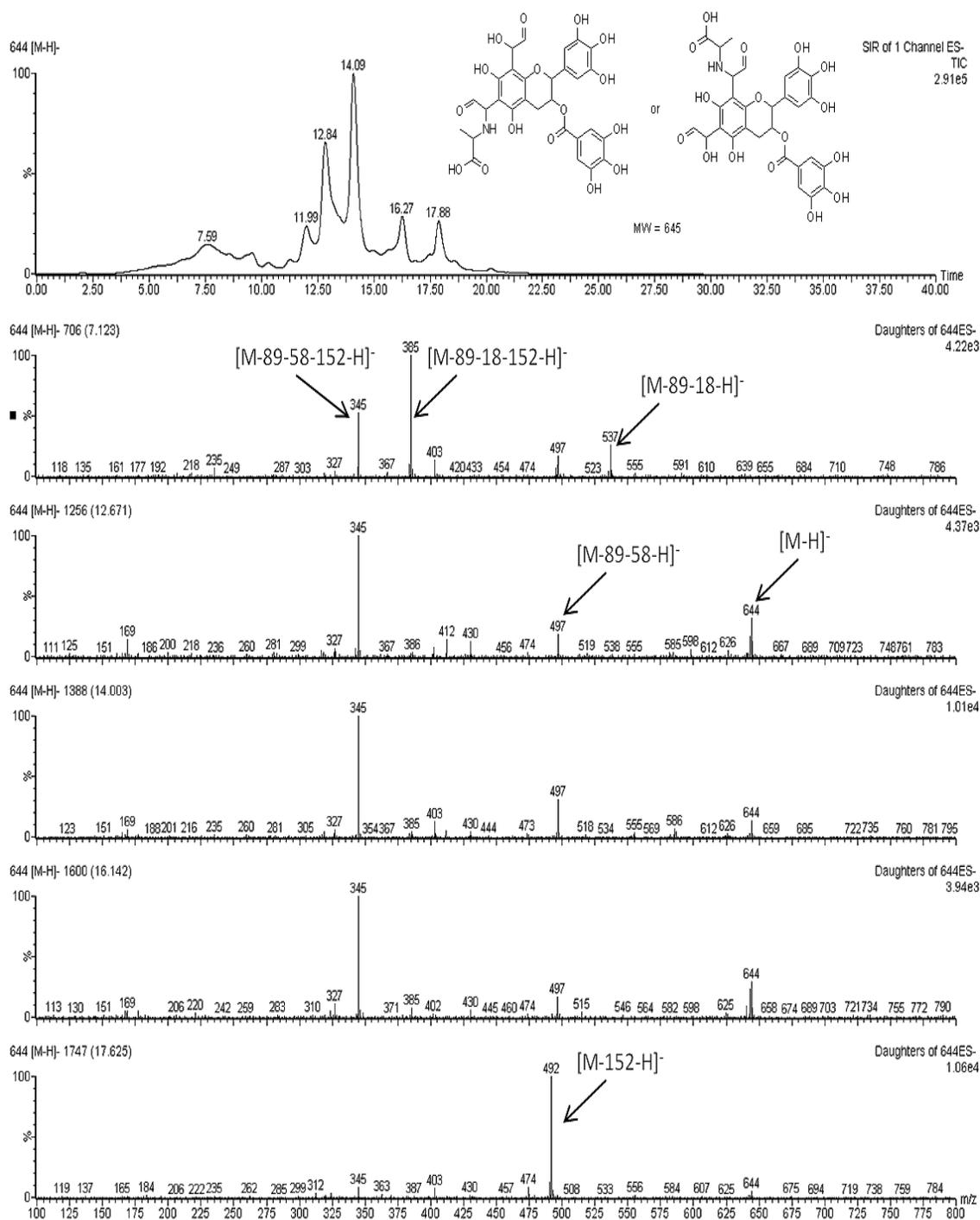
**Figure 3-5b.** Chromatograms and LC/MS/MS spectra of analyte MW 645(644 [M-H]<sup>-</sup>) generated from GO-Ala-EGCG model. The EGCG concentration was at 20 mM.
