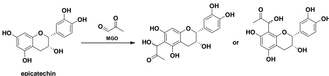
**Figure 1-2.** Epicatechin carbonyl-trapping reaction and formation of EC-MGO adduct<sup>4d</sup>.
