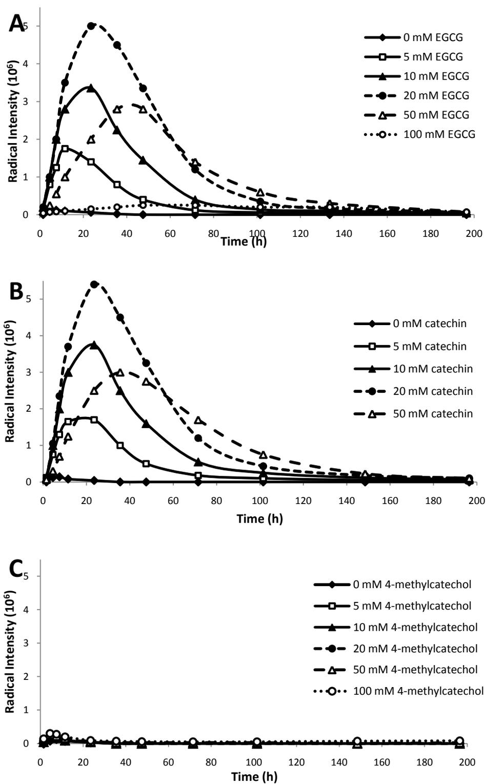
**Figure 3-1.** Effects of (a) EGCG, (b) catechin, and (c) 4-methylcatechol on the generation and fate of pyrazinium radical in GO–Ala aqueous model at 25 °C.
