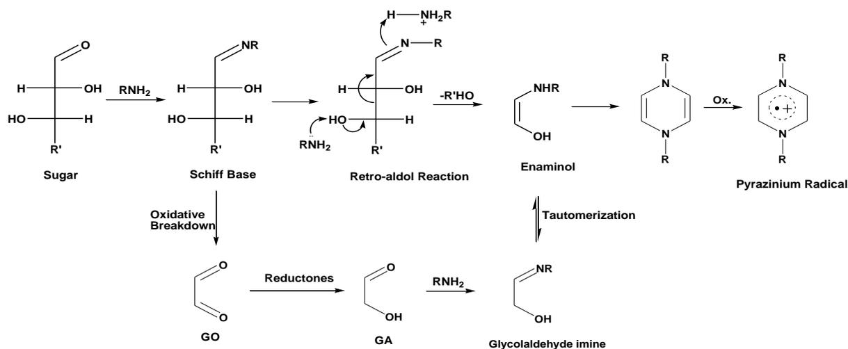
**Figure 1-1.** Mechanism of the pyrazinium radical cation formation in the Maillard reaction<sup>2-3</sup>.
