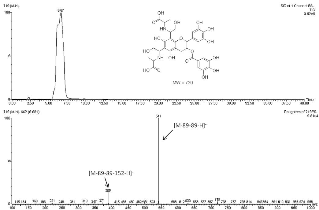
**Figure 3-11b.** Chromatogram and LC/MS/MS spectrum of analyte MW 720 ( $719 [M-H]^-$ ) generated from GA-Ala-EGCG model.
