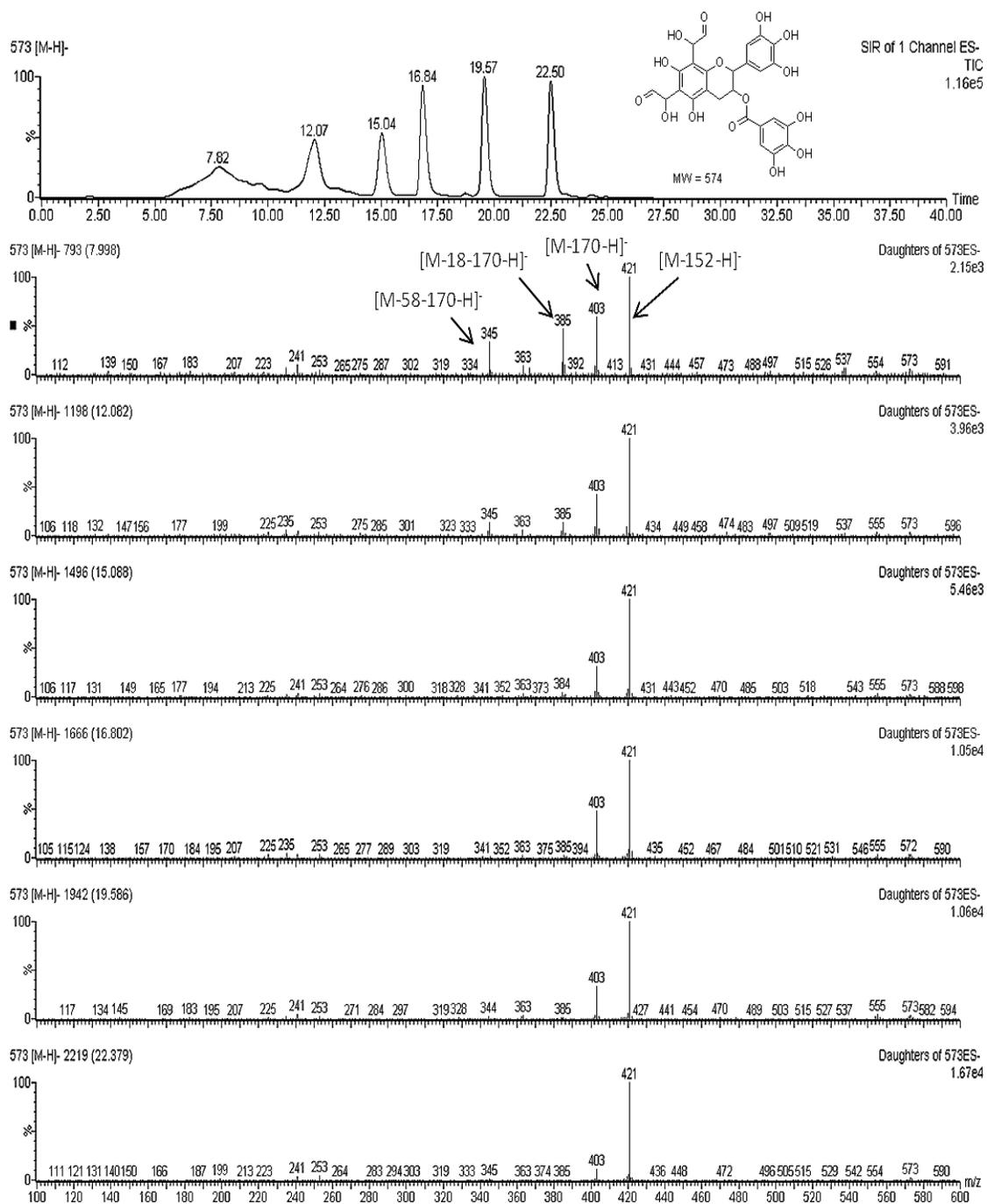
**Figure 3-4b.** Chromatogram and LC/MS/MS spectra of di-substituted EGCG-GO adduct generated from GO-Ala-EGCG model.
