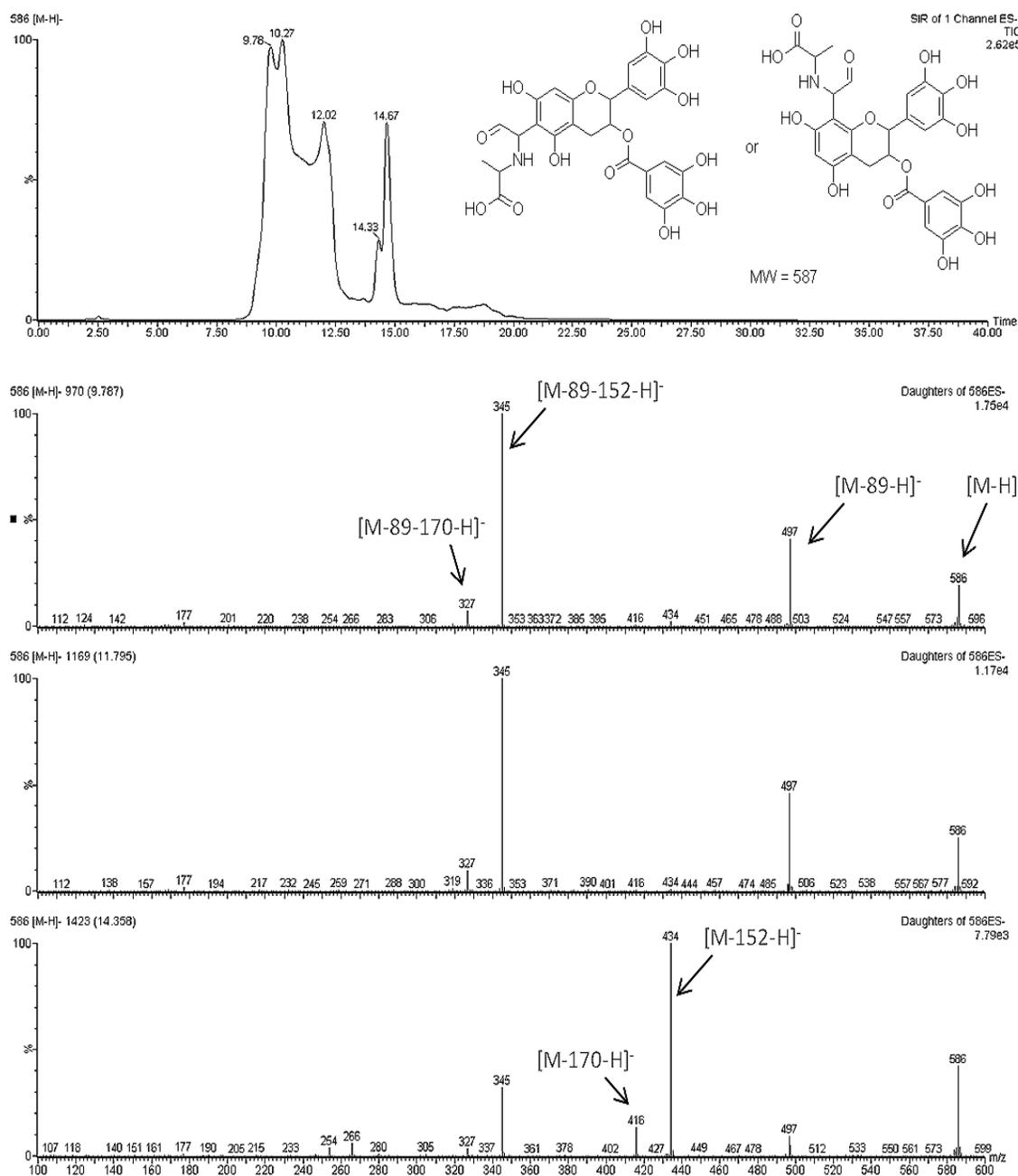
**Figure 3-5a.** Chromatogram and LC/MS/MS spectra of analyte MW 587 (586 [M-H]<sup>-</sup>) generated from GO-Ala-EGCG model. The EGCG concentration was at 20 mM.
