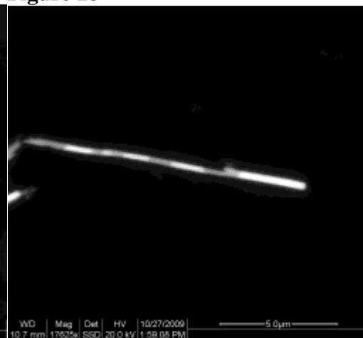
Figure 18. SEM image of the annealed Au/Ag NW after annealing.
