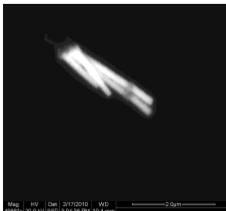
Figure 6. SEM image of Au/Bi/Au nanowires
