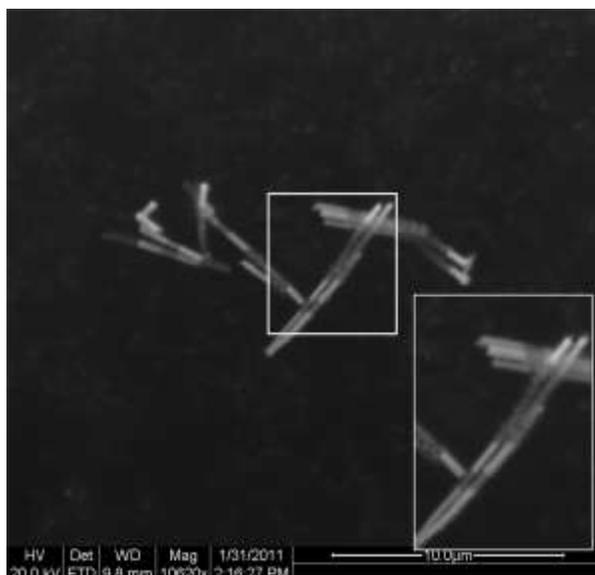
Figure 20. SEM image of the Au/Ag/Au/Ni/Au/Cu/Au NW following the  $\text{H}_2\text{PtCl}_6$  reaction.
