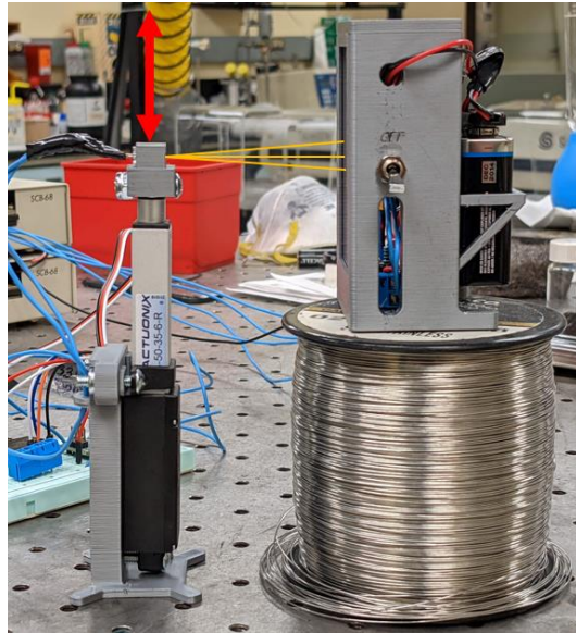
Figure 17. Test setup for photodiode instrument with linear actuator motion path (red arrow) and LED emission lines representation (orange lines).
