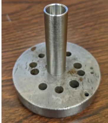
Figure 20. Propellant holder with 0.5in upper hole
