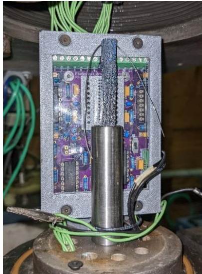
Figure 22. Photodiode amplification circuitry mounted on strand burner plug
