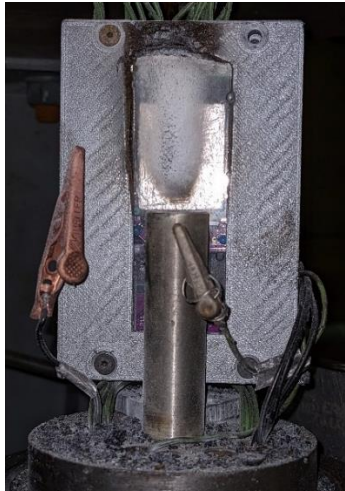
Figure 25. Photodiode quartz slide covered with exhaust products
