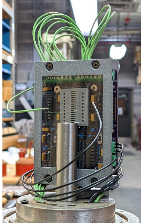
Figure 14. Circuitry holder for the photodiode array
