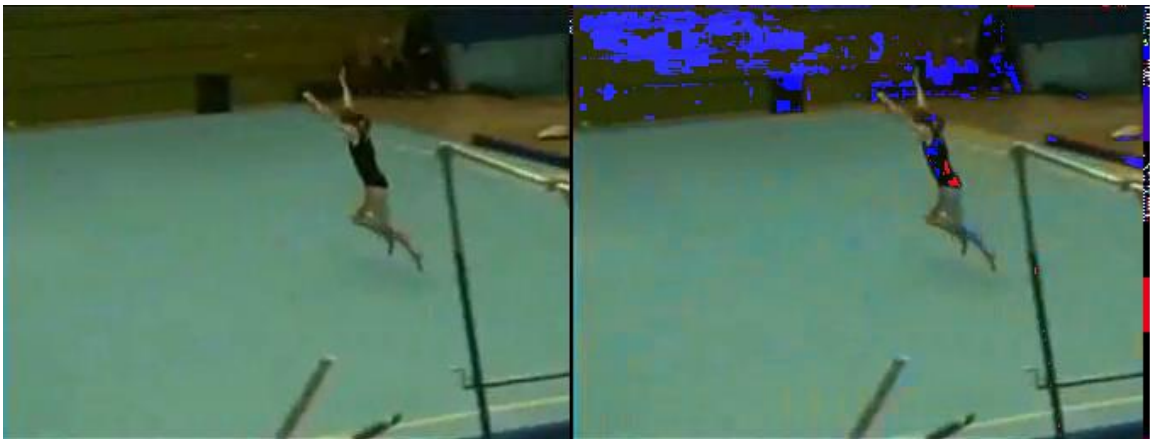
Figure 4-1: Decoder Extracted Frame (left) vs Frame Decompressed using raw MVs and Residuals (HMDB-51[21])
