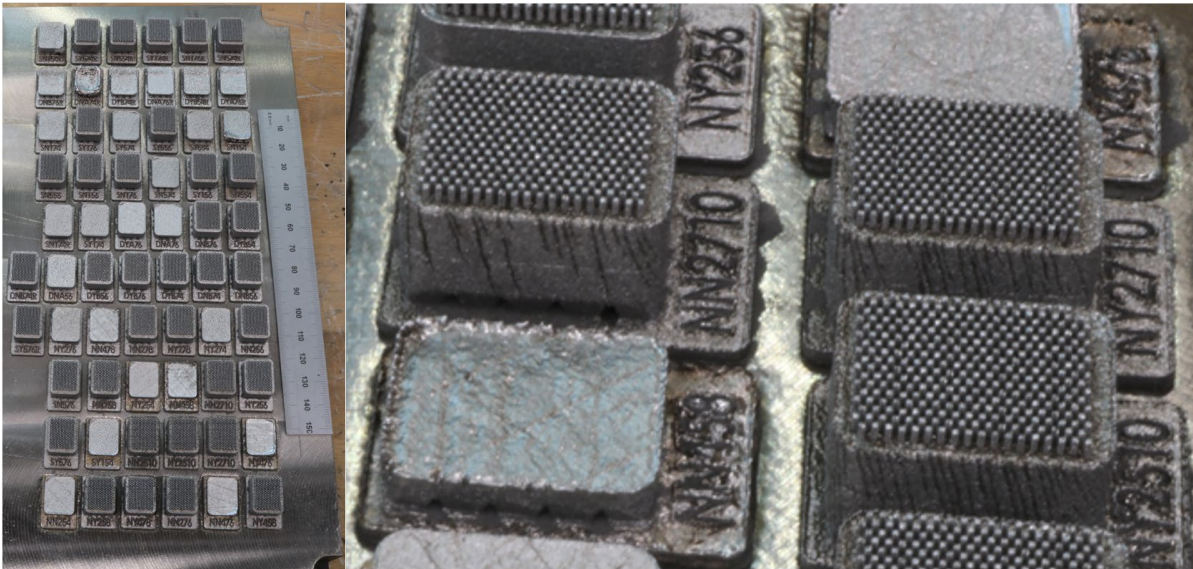
Figure 5: Image of all specimens on the build substrate (left) and a magnified image of some terminated and completed specimens (right).
