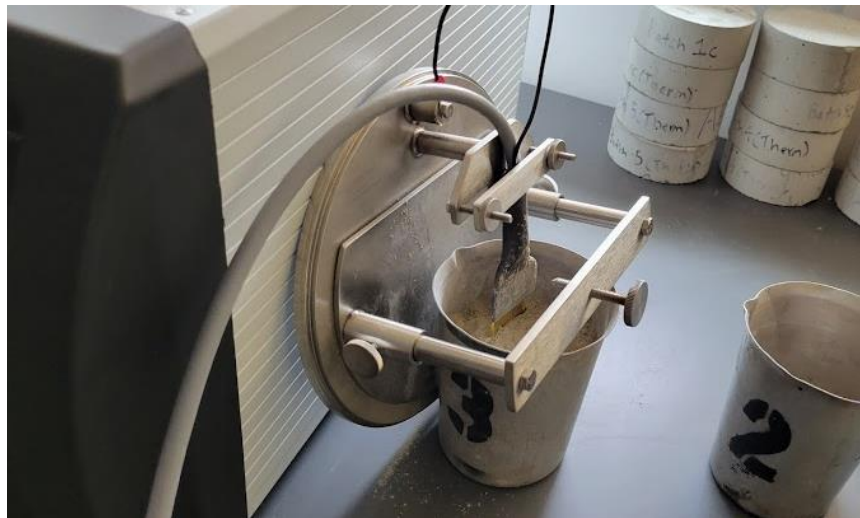
Figure 14. TPS Sensor embedded in a powder of aggregate
