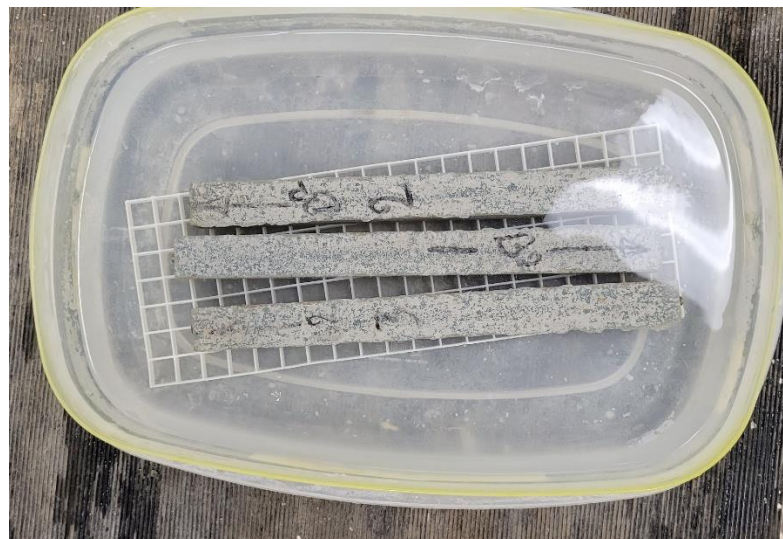
Figure 22. ASR test concrete samples
