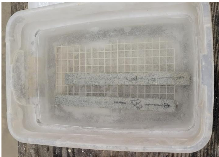
Figure 18. Mortar bars submerged in NaOH bath for the ASR test
