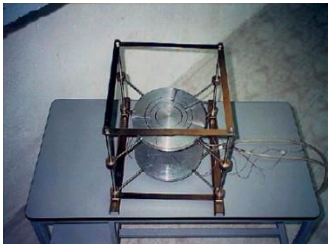
Figure 1. Guarded hot plate apparatus for measuring the thermal conductivity of insulating solid materials (Xamán et al. 2009)
