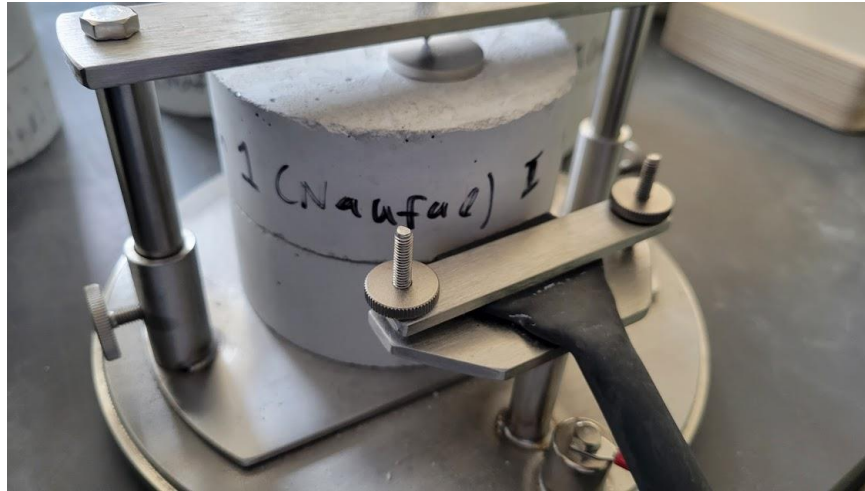
Figure 6. TPS Kapton sensor sandwiched between the sample
