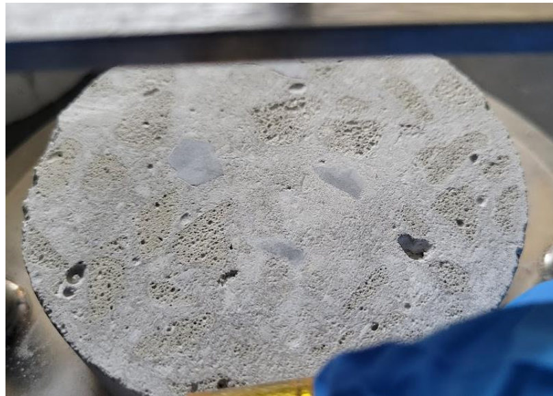
Figure 8. The exposed porous structure of the FGA is embedded in a concrete sample.
