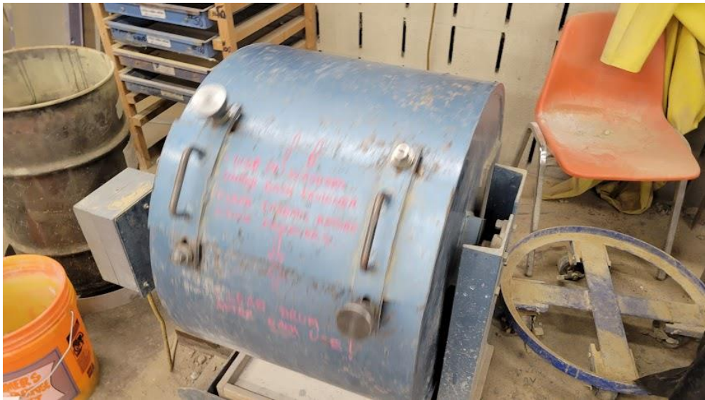
Figure 16. Los Angeles abrasion crusher machine
