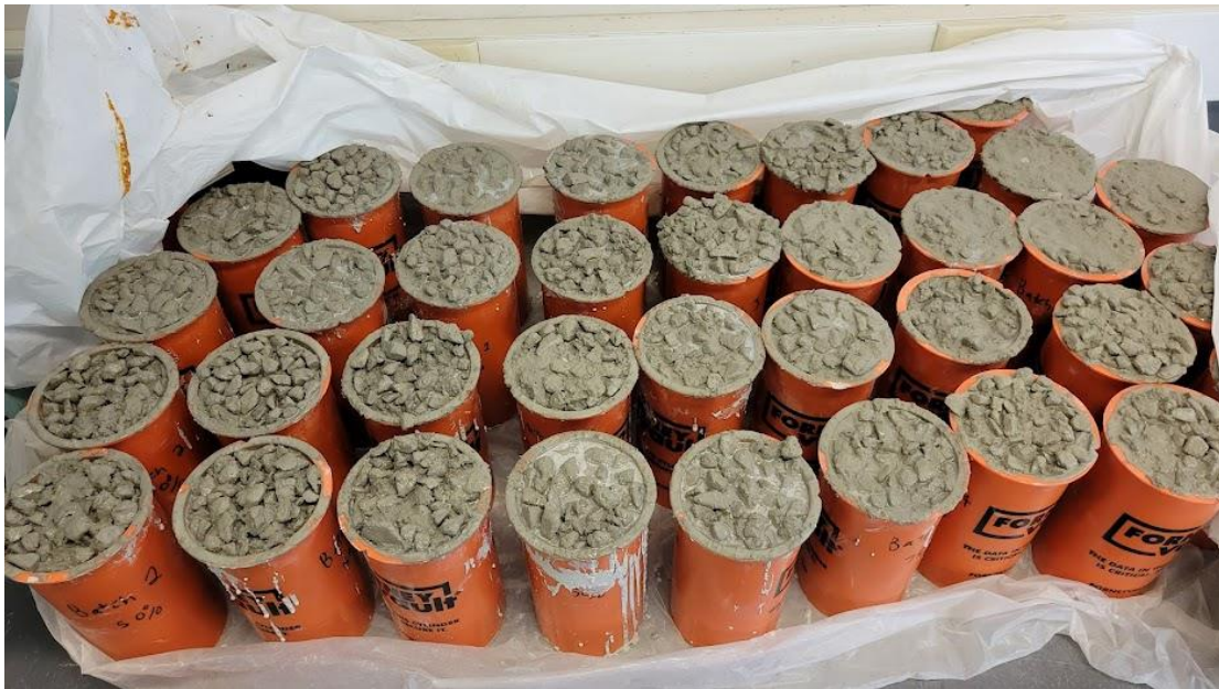
Figure 9. Batch Mixes being cast into cylinder molds
