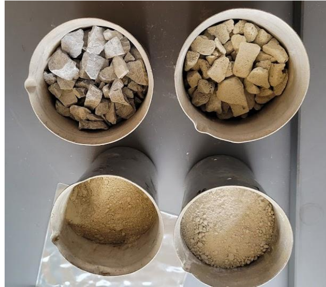
Figure 7. Dry components of improved insulation concrete, clockwise from top right: Aero Aggregate, OPC, Sandstone, Limestone Aggregate
