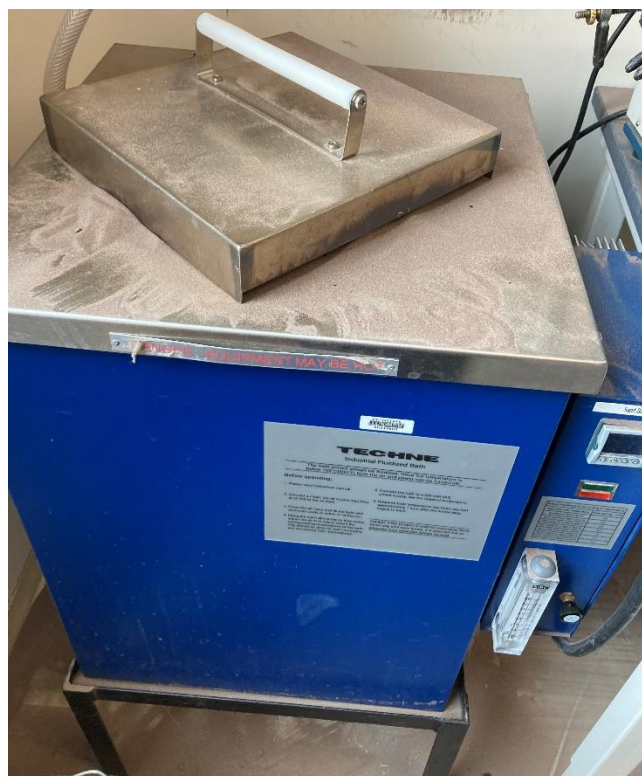
Figure 2. Techne Industrial Fluidized Sand Bath.
