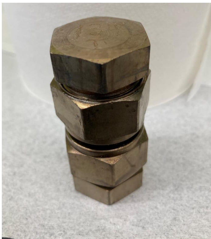
Figure 1. 10.0 mL Swagelok Batch Reactor.
