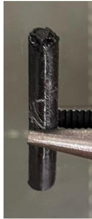
Figure 16. An example of a failed print. The layers began to shift when switching from PETG to ASA, resulting in increased surface roughness. The part finished printing, but the top of the part is extremely rough and uneven due. More extreme failure cases experienced ASA layers no longer adhering when layer shifting becomes too great.
