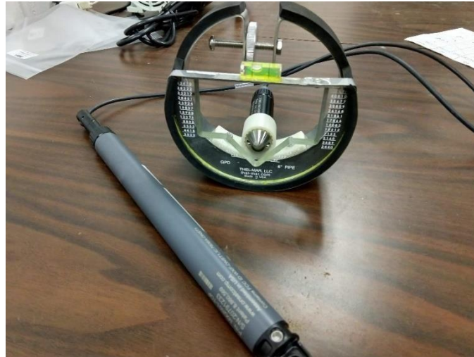
Figure 2.2 Onset HOB0 MX2001 Bluetooth pressure transducer and Thel-Mar pipe weir
