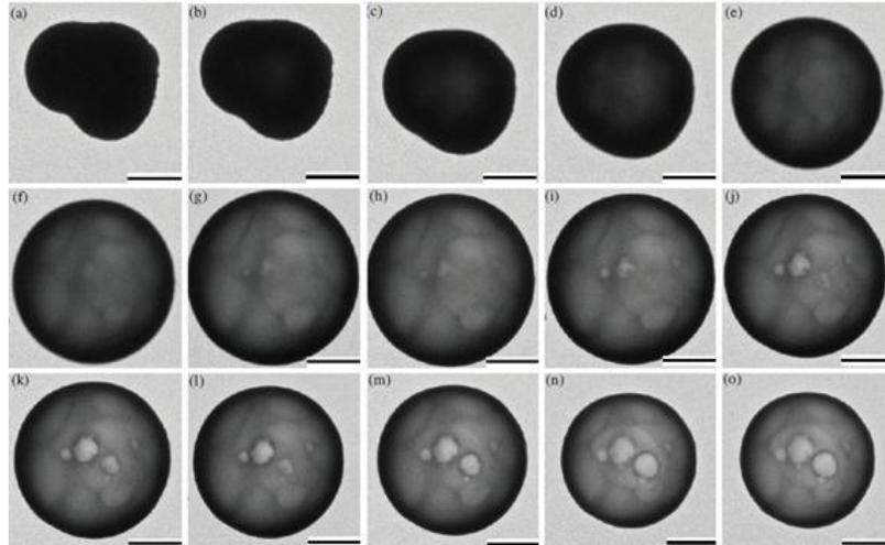
**Figure 17 Growth of particle while exposed to 120 keV TEM beam for durations of (a) 0.6, (b) 0.8, (c), 0.9, (d), 1.26, (e) 1.4, (f) 1.5, (g) 1.6, (h) 2, (i) 2.4, (j) 2.9, (k) 3.3, (l) 4.43, (m)8.7, (n)11.2, (o) 12.5 s**
