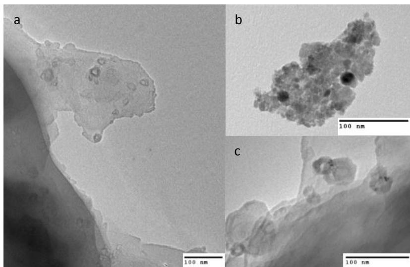
**Figure 5 (a,b,c) TEM images taken of product from reactor wall with 15 W plasma with 5 minute experimental duration**
