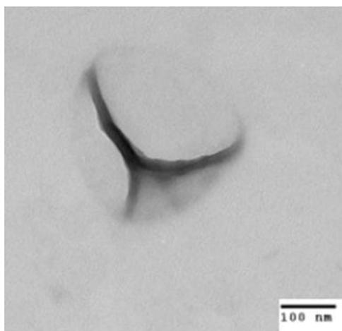
**Figure 23 TEM image of nanoparticle after UV exposure**
