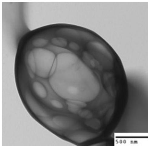
**Figure 20 TEM image of stabilized nanoparticle after exposure to 60 mW HeNe laser and electron beam**
