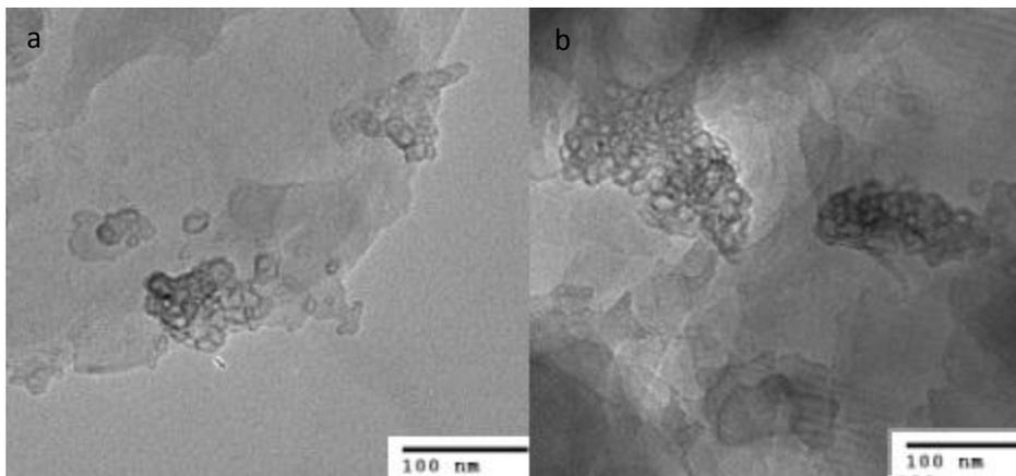
**Figure 6 (a,b) TEM images taken of product from reactor wall with 15 W plasma and 20 minute experimental duration**
