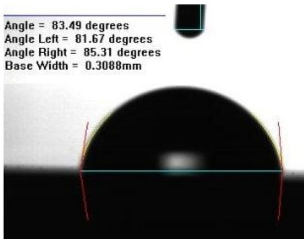
**Figure 15 Contact angle between heptane based deposition and wafer**
