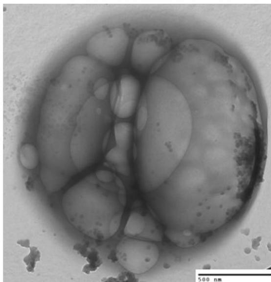
**Figure 21 TEM image of nanoparticle after exposure to 100 mW Ar laser**
