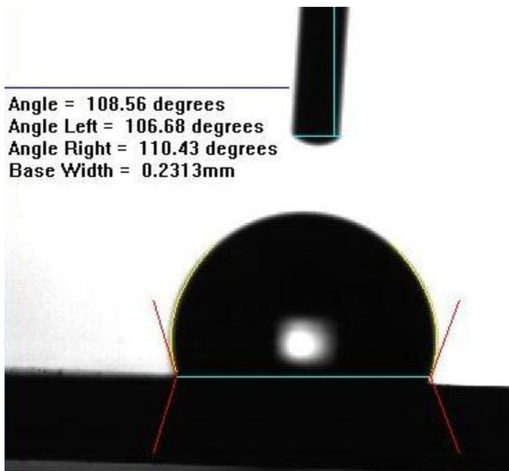
**Figure 13 Contact angle measurement between water and silicon wafer**
