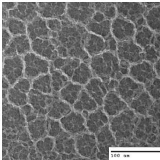
**Figure 11 TEM image taken of product from reactor wall with 50 W plasma and 30 minute experimental duration**
