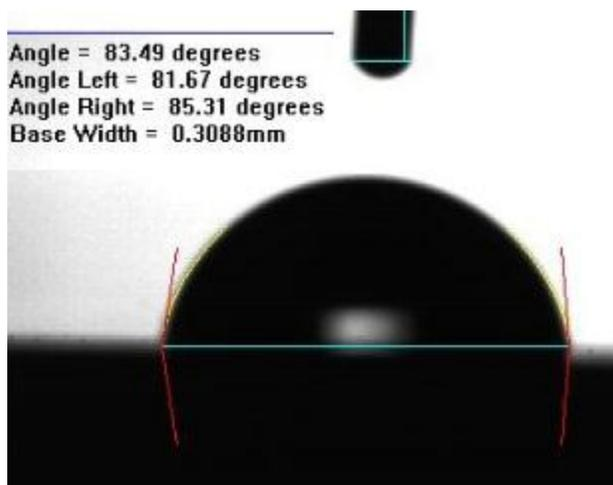
**Figure 14 Contact angle between toluene based deposition and wafer**
