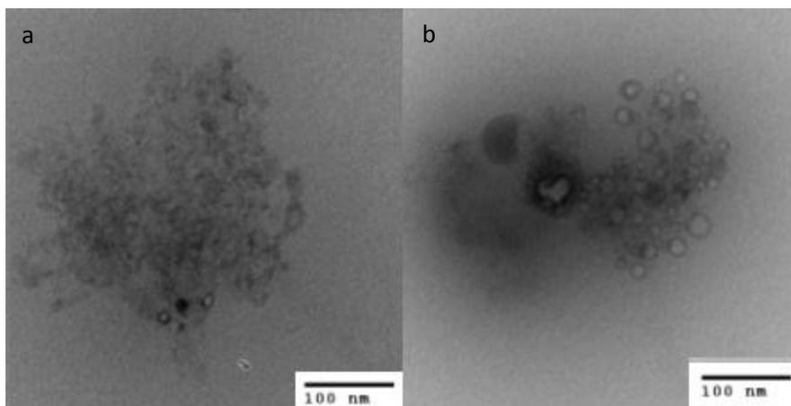
**Figure 7 (a,b) TEM images taken of product from reactor wall with 40 W plasma and 5 minute experimental duration**
