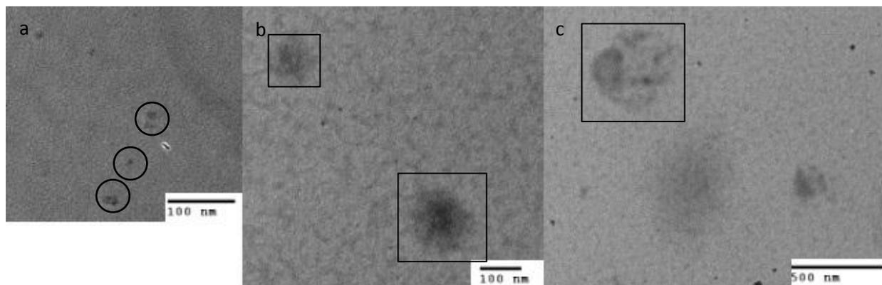
**Figure 8 (a,b,c) TEM images taken of product from reactor wall with 40 W plasma and 20 minute experimental duration**
