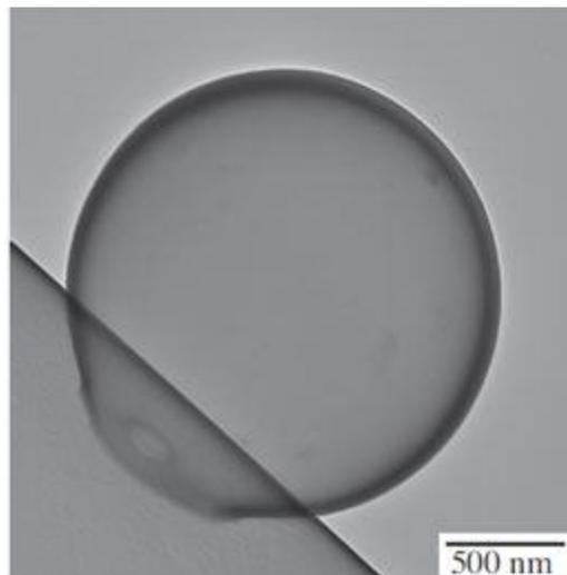
**Figure 18 TEM image of hollow particle attached to the carbon film on the TEM sample holder**
