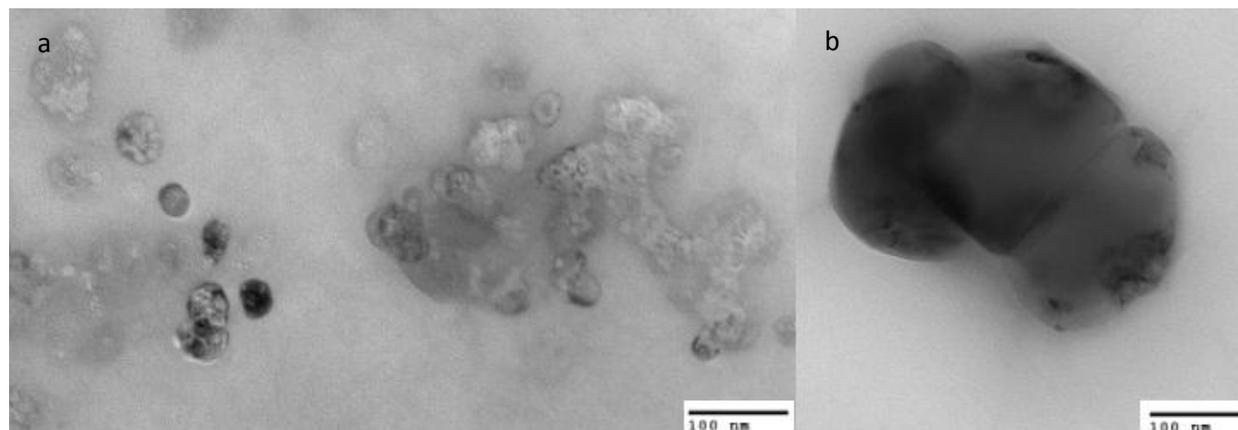
**Figure 9 (a, b) TEM images taken of product from reactor wall with 40 W plasma and 27 minute experimental duration**
