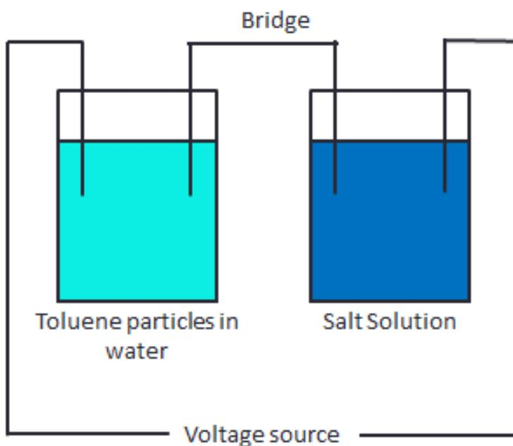
**Figure 4 Voltage testing setup**
