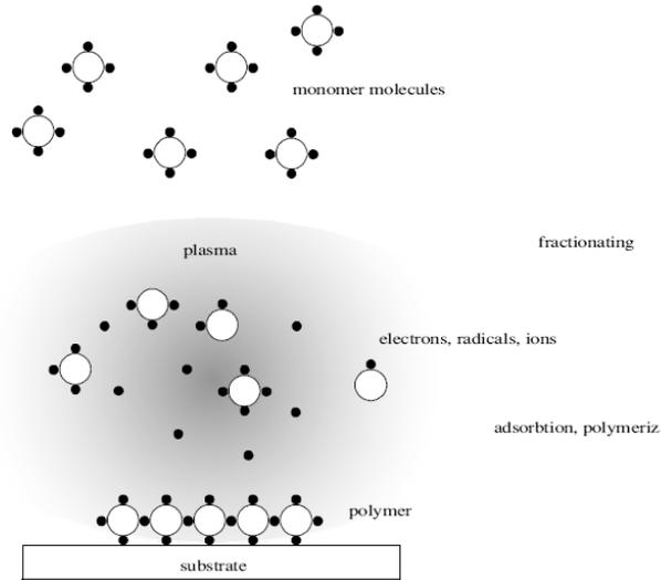
**Figure 1 Formation of polymer product from monomer molecules (2)**
