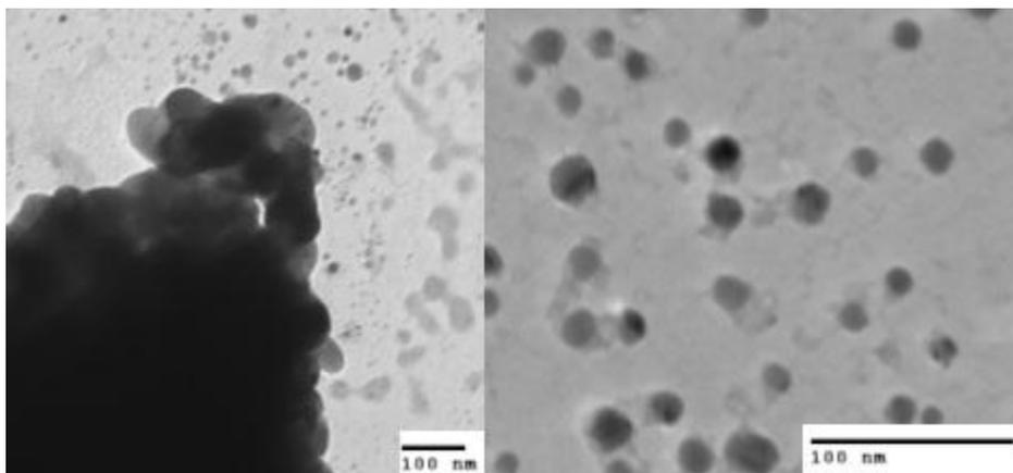
**Figure 24 TEM image of particles after applying 5 V to the sample**
