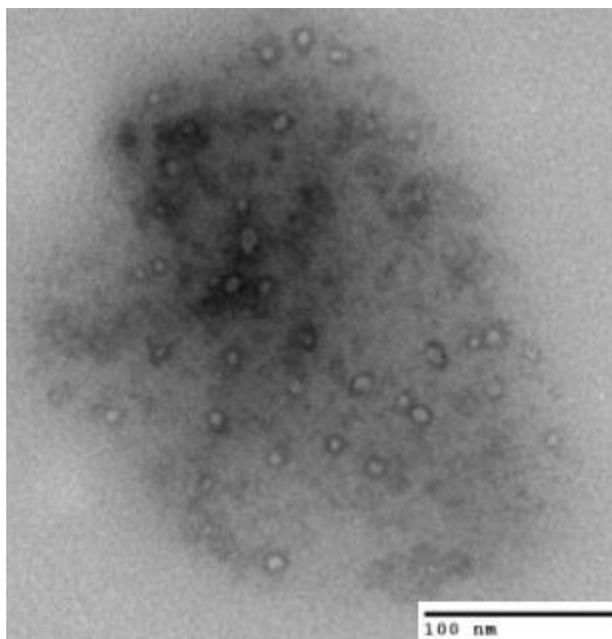
**Figure 10 TEM image taken of product from reactor wall with 60 W plasma and 20 minute experimental duration**
