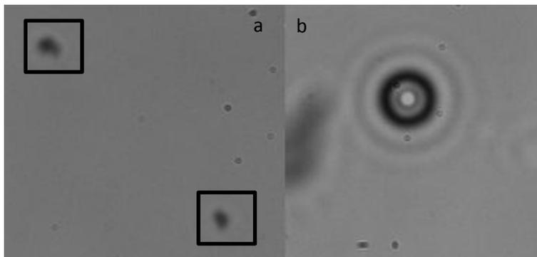
**Figure 19 Nanoparticles under light microscope a) before TEM exposure b) after TEM exposure**
