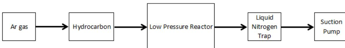
**Figure 2 Block flow diagram of experimental setup**
