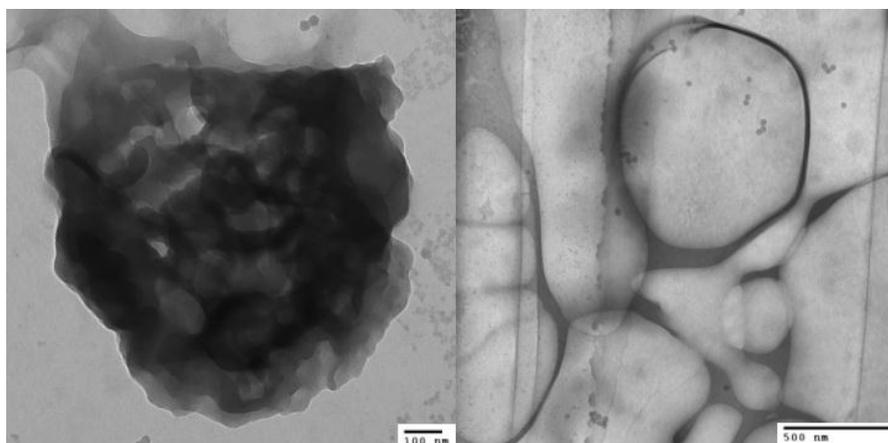
**Figure 22 TEM image of a) cluster of particles stabilized under 200 mW Ar laser exposure
