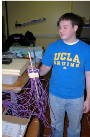
Figure 3.11 Thermocouples were bundled together to be put in the ice bath to minimize the influence of spatial temperature differences in the water.
