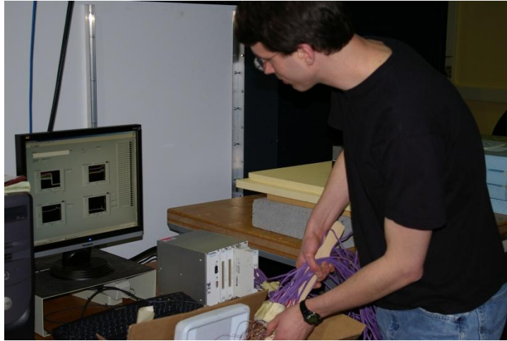
Figure 3.13 The bundle of thermocouples were inserted to the ice bath multiple times for two to three minutes to allow for equilibrium.
