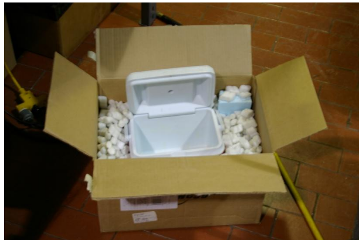
Figure 3.12 The ice bath was inside of a cooler with insulation surrounding it to ensure a temperature as close as possible to 0°C.
