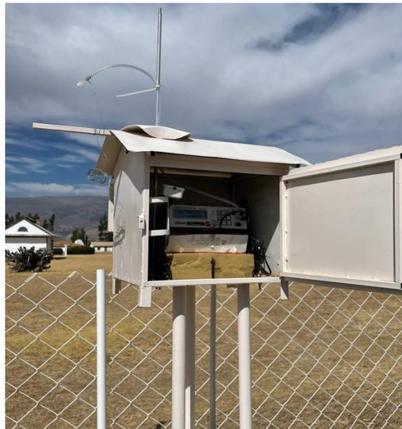
**Figure 19: Grimm Portable Dust Monitor installed at HYO**
