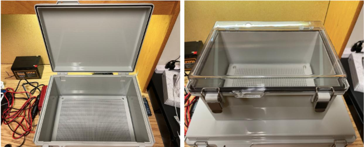
**Figure 26: Photographs of larger (left) and smaller (right) Gratury junction boxes**
