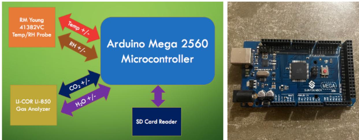
**Figure 23: Data logging system diagram with Arduino Mega 2560 microcontroller**
