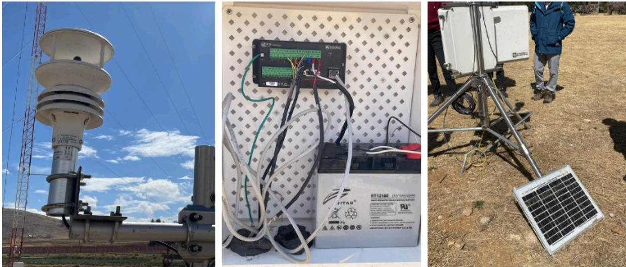
**Figure 18: HYO weather station (left) along with its data logger, power supply, and solar battery charger**
