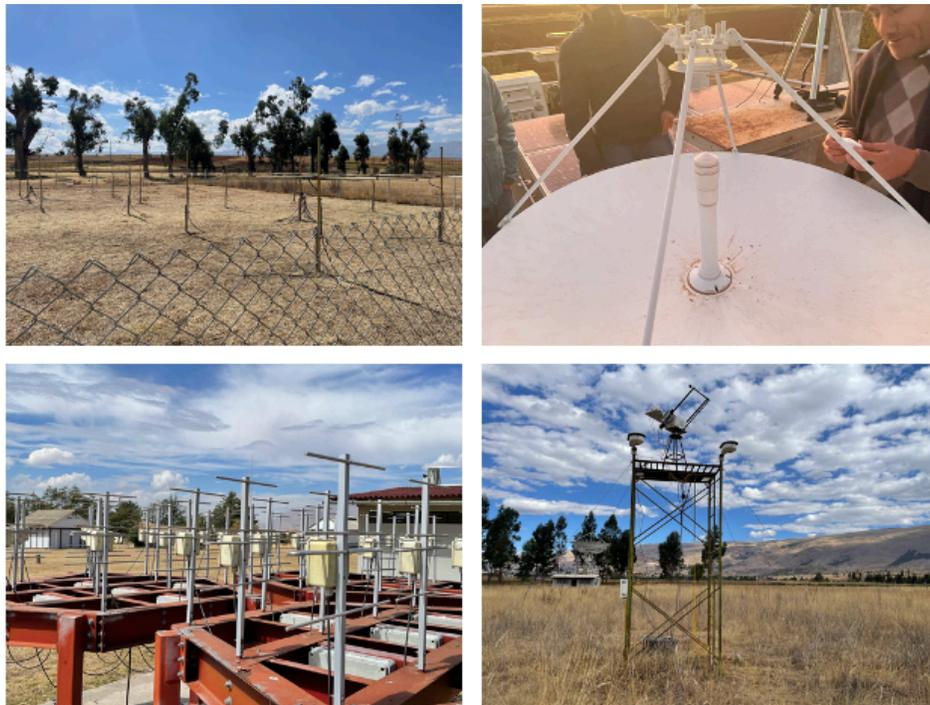
**Figure 20: HYO radar and radiation devices (clockwise from top left): Boundary Layer and Troposphere Radar (BLTR); Ka-band Doppler radar MIRA-35c; radiation instrumentation tower; rainfall estimation radar**
