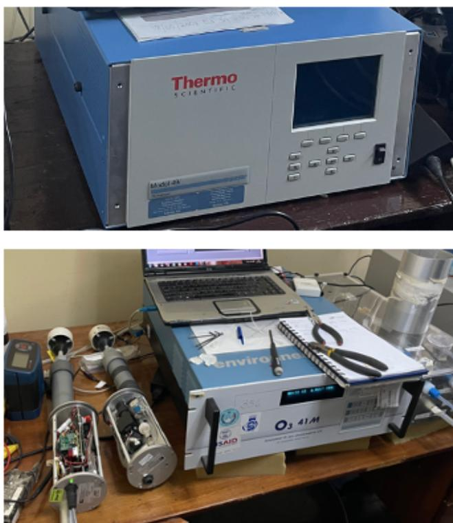
**Figure 21: Thermo Scientific 49i and Model 41M ozone analyzers at HYO**
