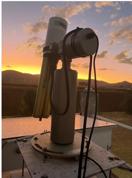
**Figure 17: Sun Sky Lunar Multispectral Photometer CE318-T installed at HYO**
