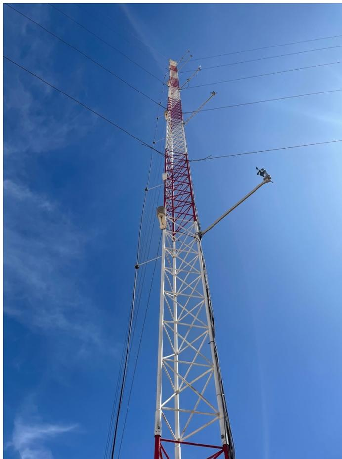
**Figure 13: Gradient Tower at HYO, measuring temperature and relative humidity**
