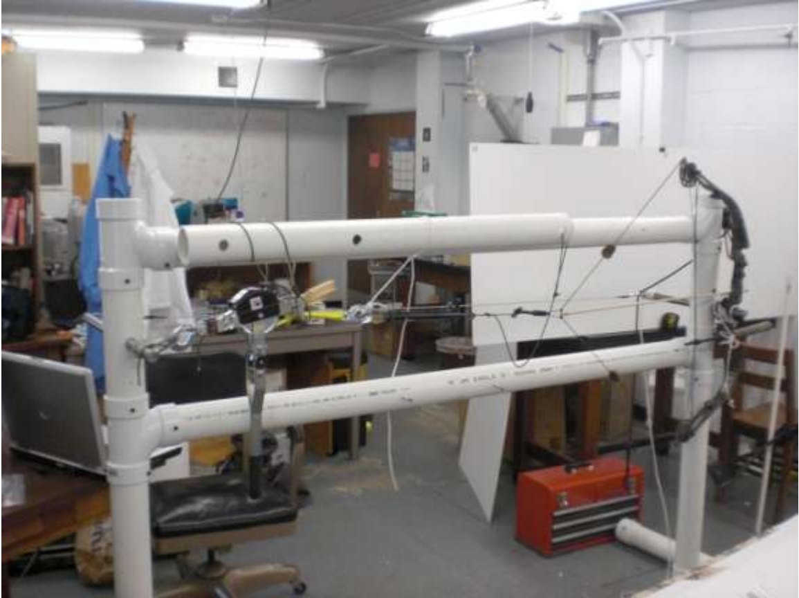
FIG. 4. A photograph of the shooting machine used during the experiments.
