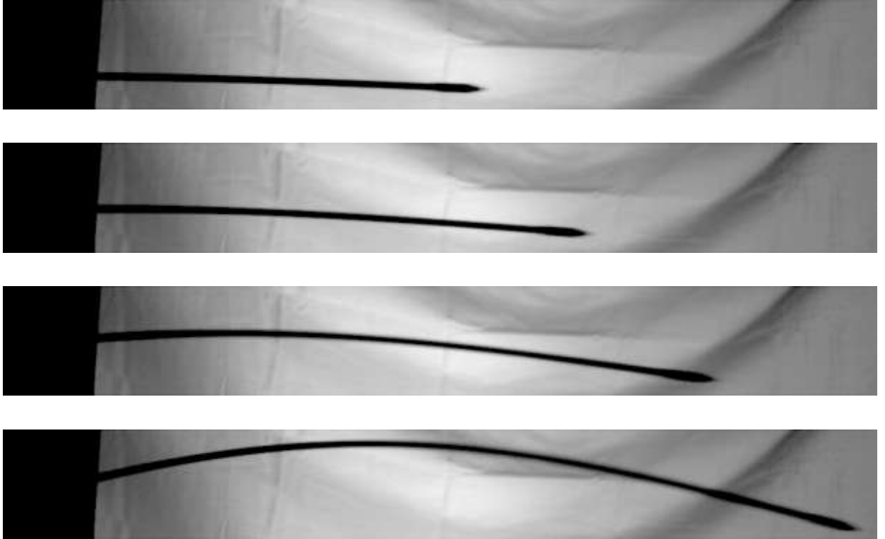
FIG. 8. The extreme buckling of a carbon arrow with a very massive tip, flying from the left to the right.
