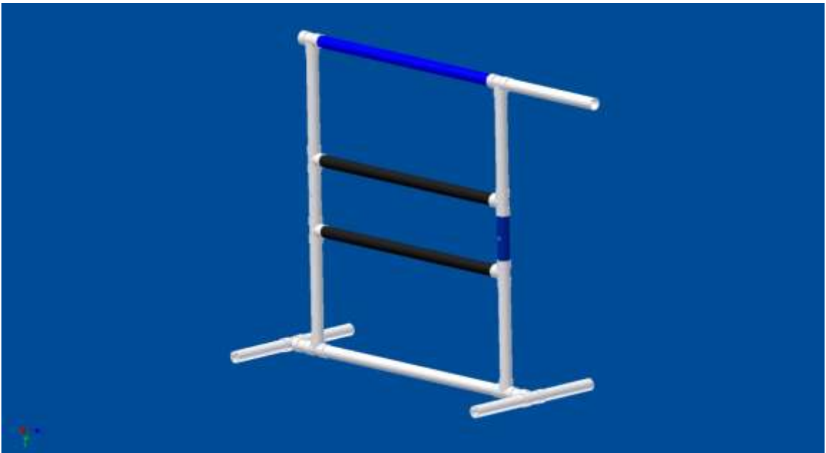
FIG. 3. A blueprint, courtesy of Robert Geist, showing the design for the shooting machine’s frame.
