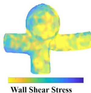
Figure 3. Colorized plot of WSS on geometry.
