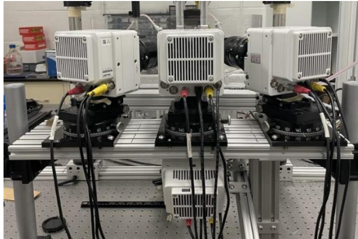
Figure 6. Four cameras are positioned to triangulate particle position within aneurysm.
