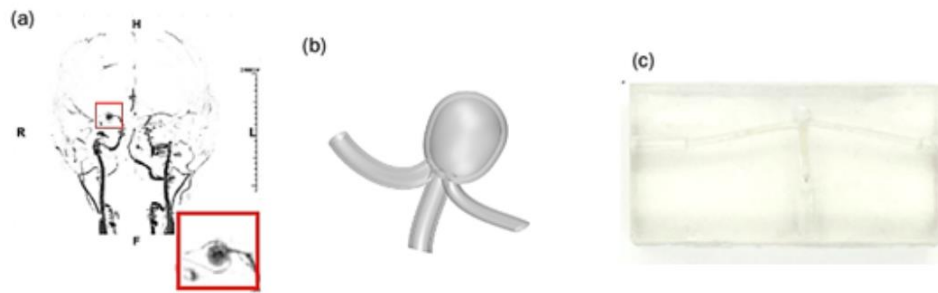
Figure 4. Manufacturing the idealized geometry. A) patient scan B) idealized CAD model C) PDMS idealized model.
