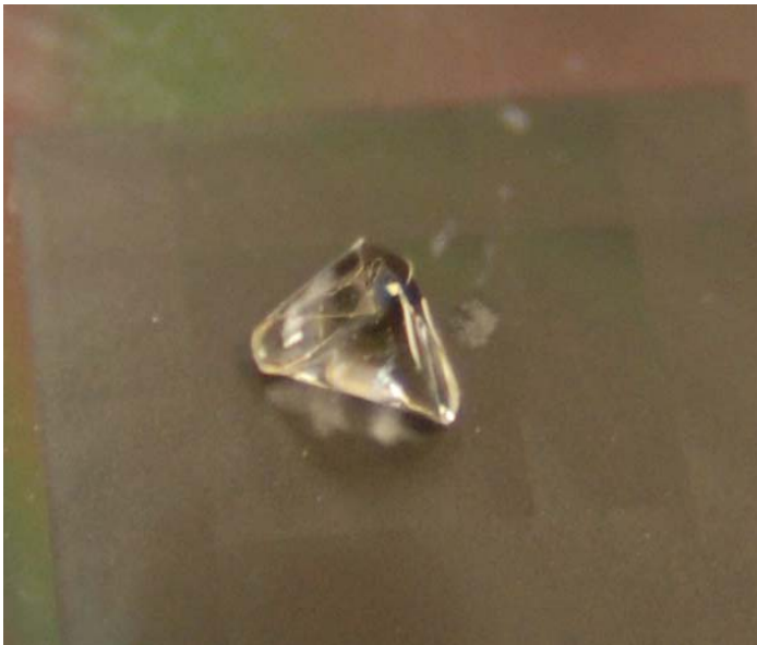
Figure 8 – Completely folded triangular PDMS sheet. The three corners of the triangle fold upward toward the central axis to form a pyramid shape.
