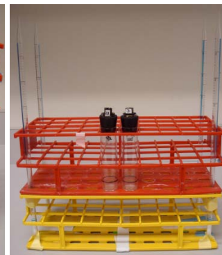
Figure 17. Drop Apparatus used to disorient flies (A) before drop and (B) after drop
