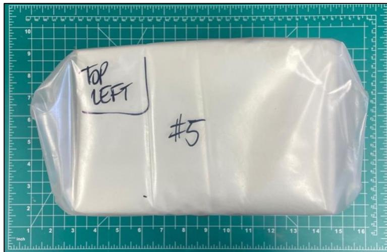
**Figure 3. Wrapped Sample of Cellular Glass**
