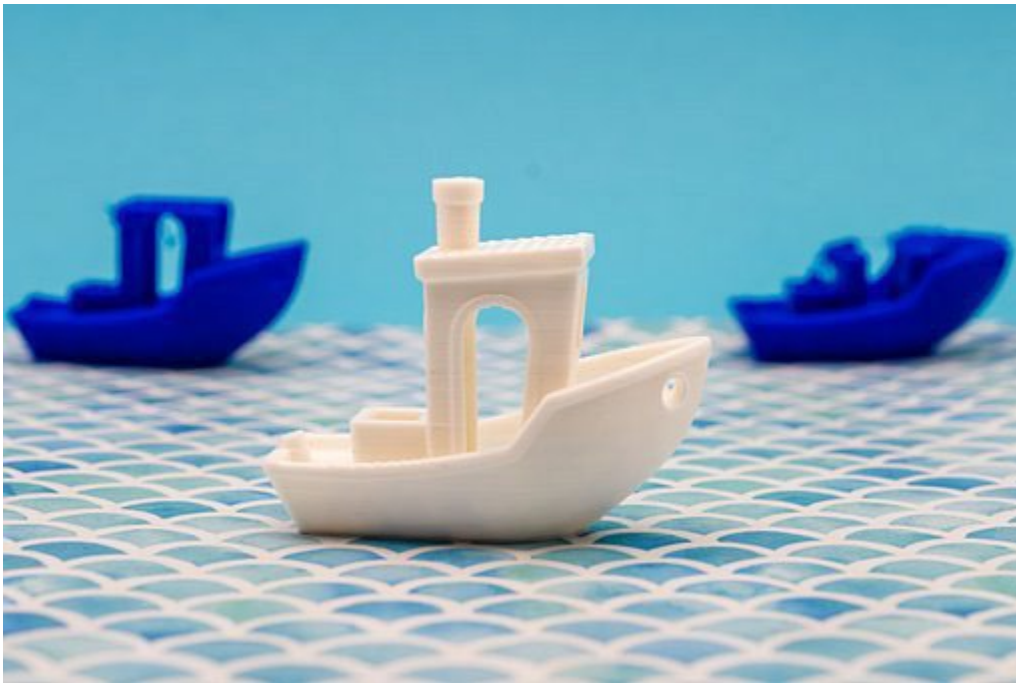
Figure 10: Plastic boats made using additive manufacturing.
