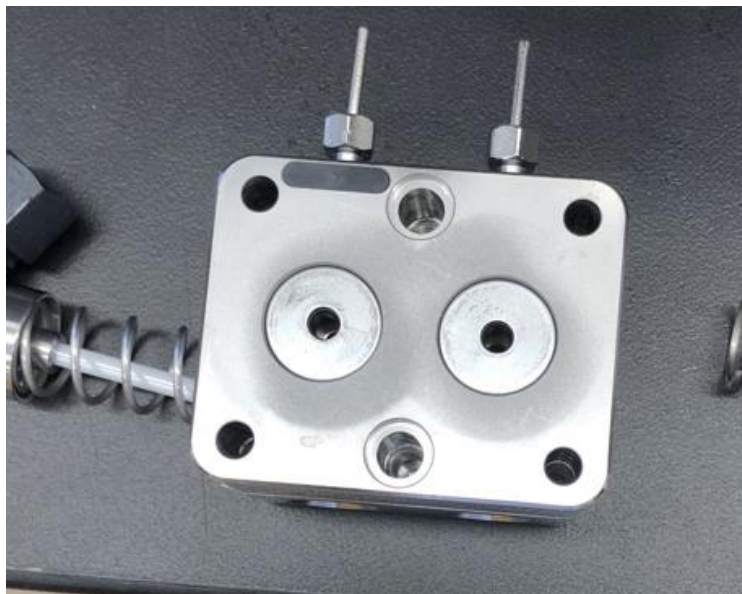
Figure 22. Aligned pump casing
