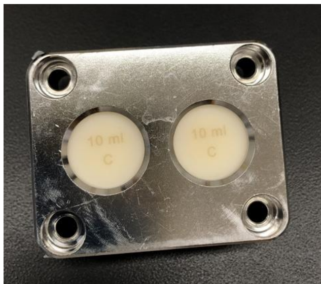
Figure 20. Alignment of plastic inner pump within metal casing
