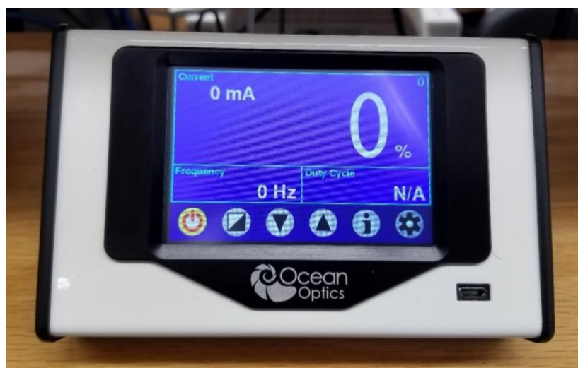
Figure 9. The LED source controller for fluorescence spectroscopy.
